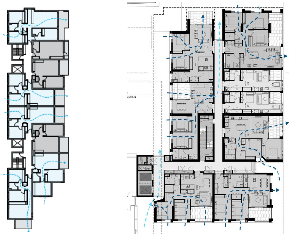
Image 1: Potential Natural Cross Ventilation Flow Paths One Approach noted in the ADG (Left), Proposed Floor Plan (Right)
