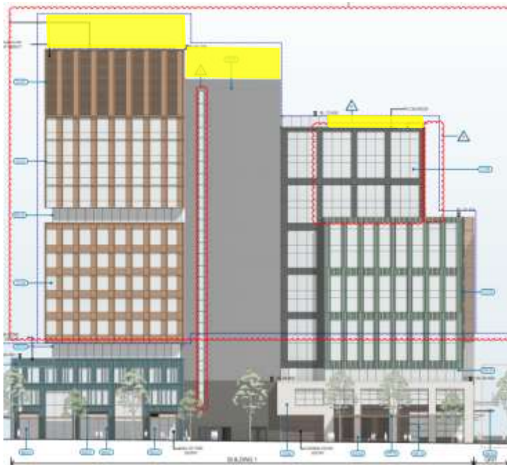
Figure 5: Western elevation (Botany Road) – amended Sheet No. WMQ-BLD1-WBG-AR-DRG-DA121 Rev F dated 15/3/21 by Woods Bagot Revised stepped Building Heights now: RL 84.1; RL 78.9; RL 70.6 (approximate difference shown in yellow shading)
