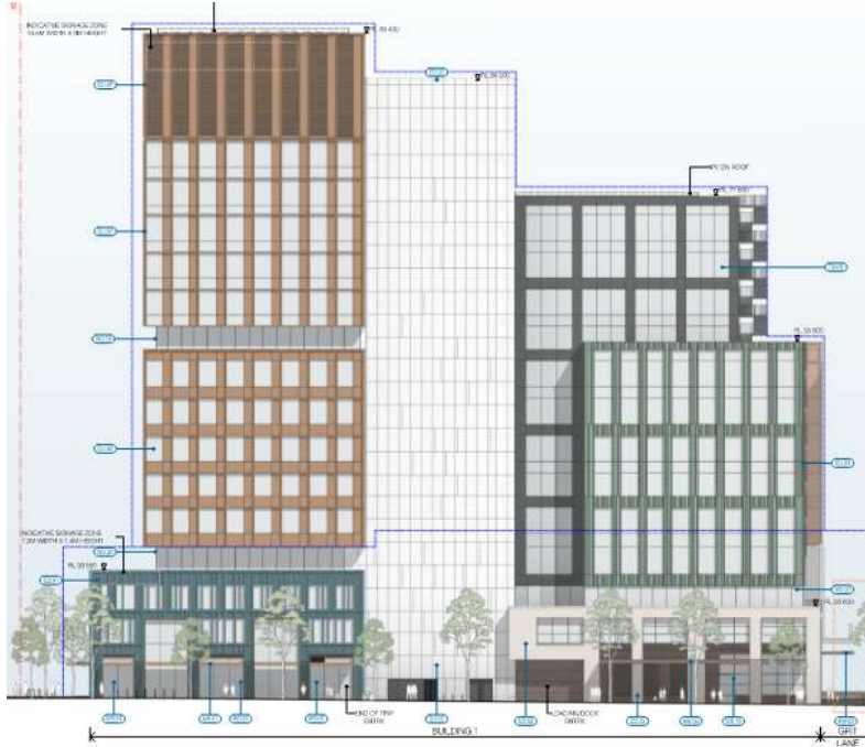
Figure 4: Western elevation (Botany Road) – as submitted (Sheet No. WMQ-BLD1-WBG-AR-DRG-DA121 Rev C dated 28/8/20 by Woods Bagot Various Building Heights as per Blue Line: Planning Envelope profile: RL 89.4; RL 84.2; RL 71.6
