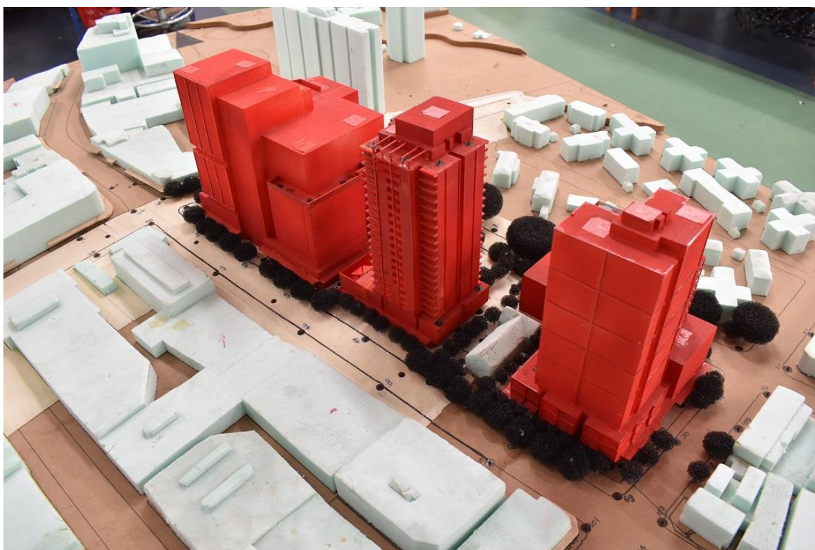
Figure A-8 – Wind Tunnel Model of Detailed Design with Mature Landscaping (View from the North-East)
