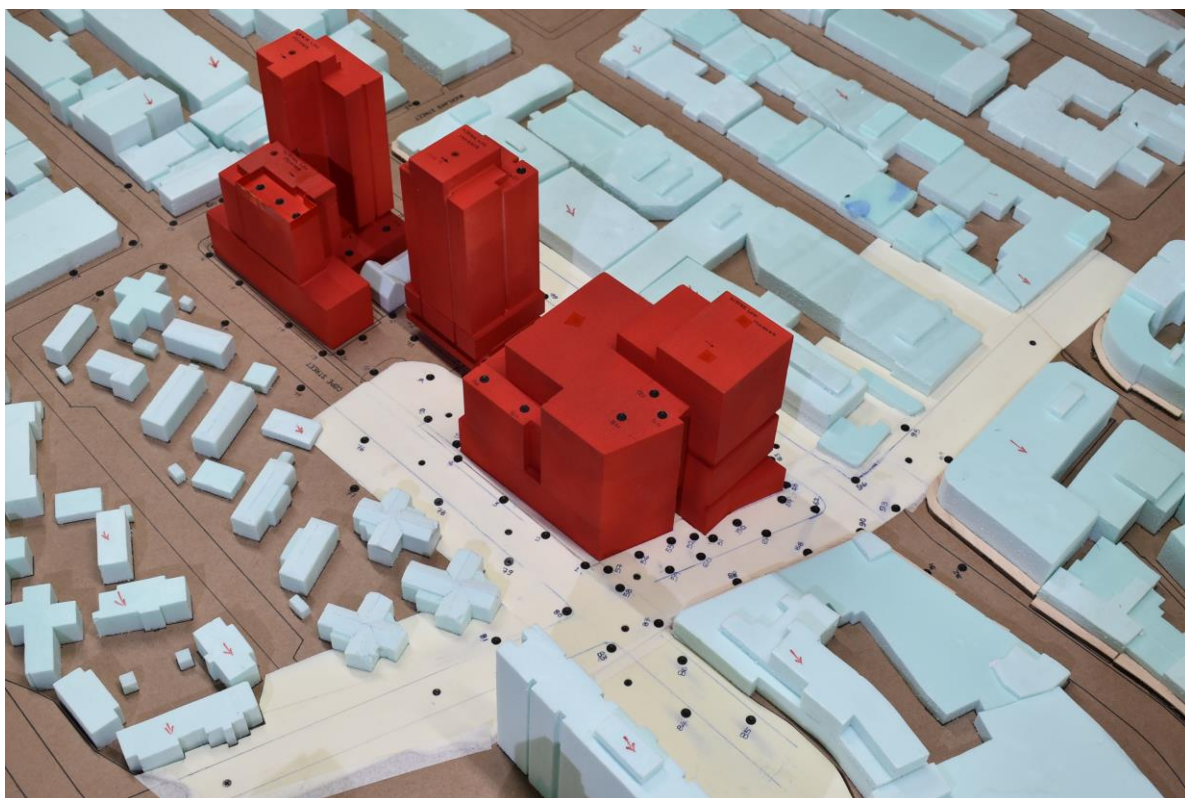
Figure 6 – Wind Tunnel Study Model – Amended DA Envelope Design Scheme
