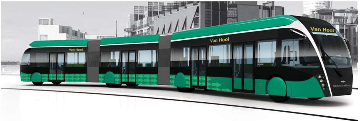
**15 CNG-fueled, 78-foot ExquiCity 24 hybrid buses by Belgium's Van Hool for BRT service in Malmo, Sweden will have new Euro6 MAN engines, series hybrid electric drivelines by Siemens, and Type III carbon fiber-on-aluminum fuel cylinders by Luxfer-Dynetek.**
