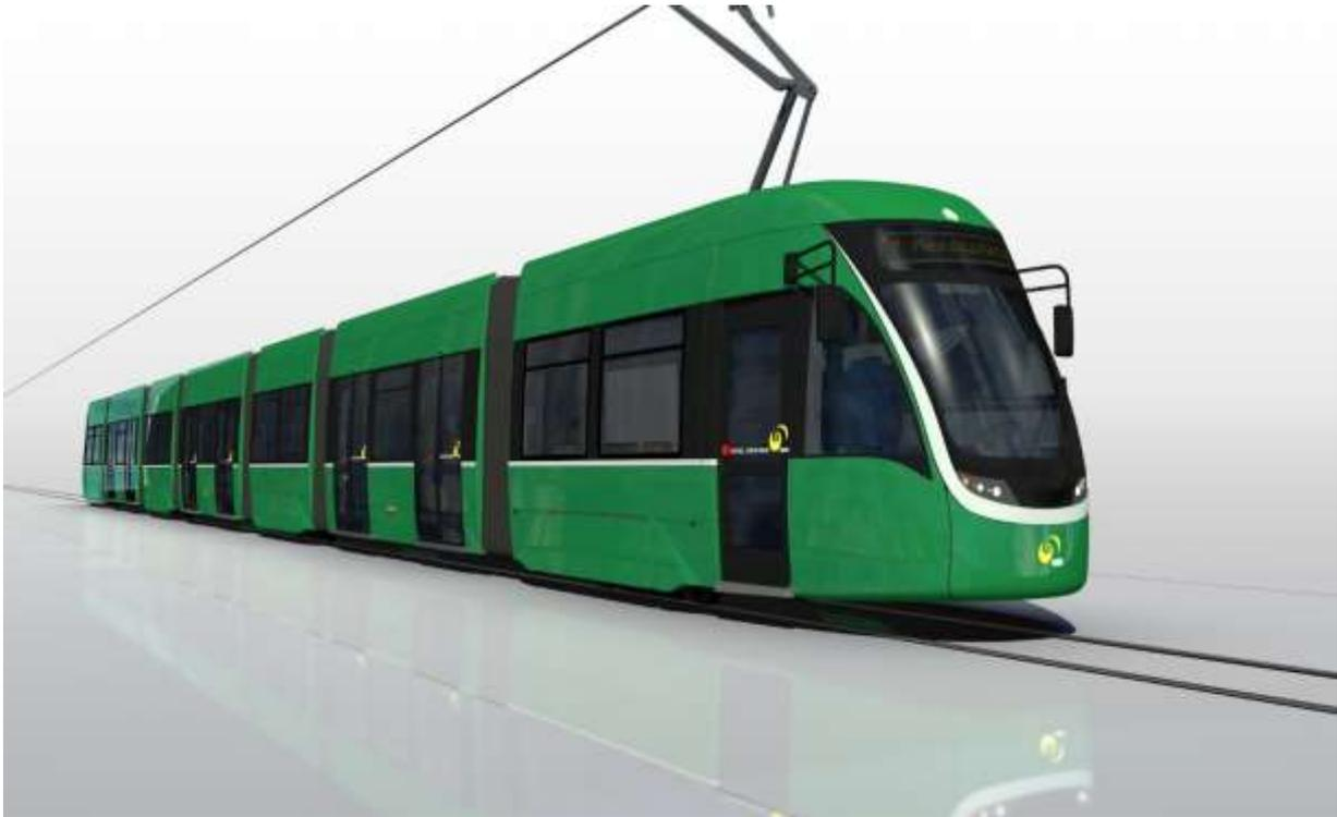
**Figure E1 – Bombardier Flexity 2 conventional tram – same model as Gold Coast tram**
