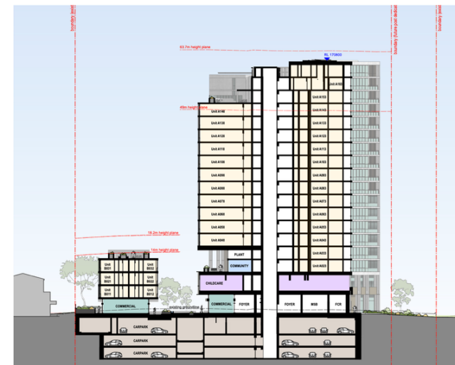
Figure C-9.1: Site Section demonstrating transitional heights across the development
