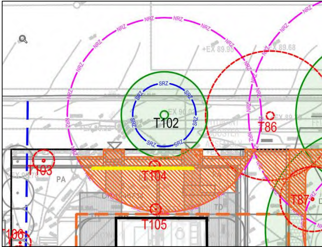
Figure 20 – Location of exploratory root mapping investigation (yellow line) within NRZ of Tree 102.
