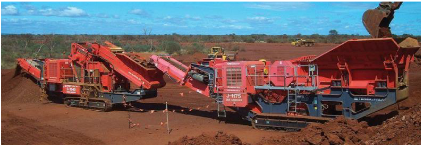
Figure 6-5 Example of a mobile crushing and screening plant process as proposed for use within the earthwork material sites
