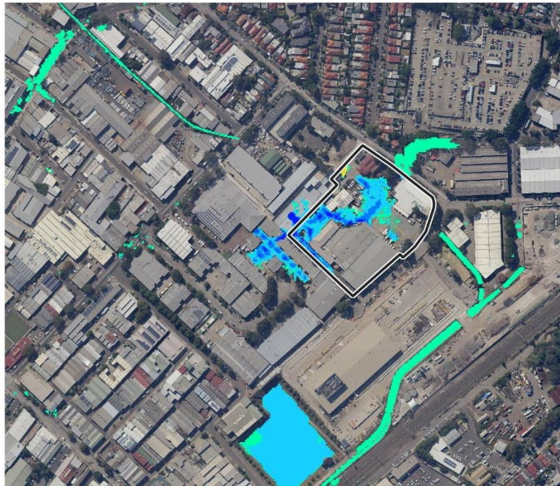
Figure 39 Post Development change in 2yr ARI flood depth (m)
