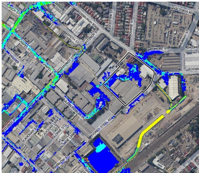
Figure 9 Pre Development 2yr ARI Flood Velocity (m/s)
