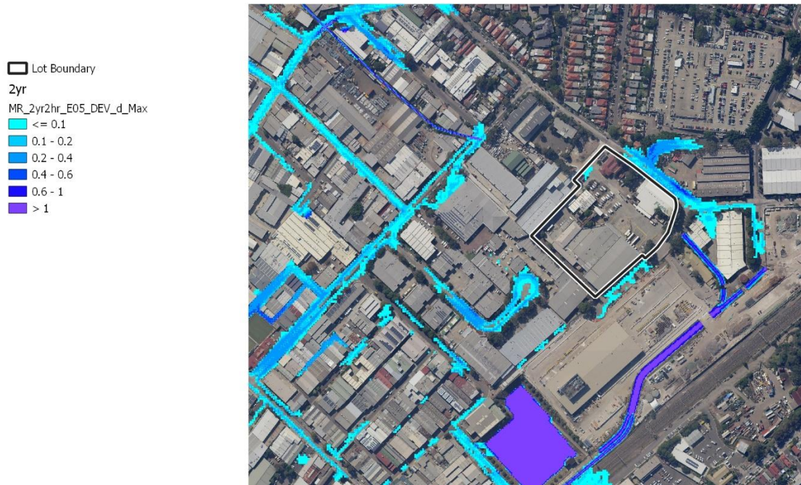
Figure 23 Post Development 2yr ARI Flood Depth (m)
