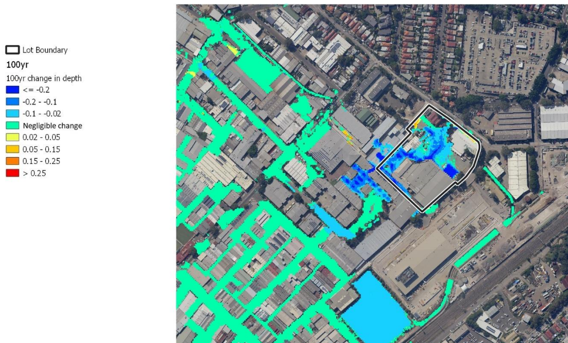
Figure 42 Post Development change in 1% AEP flood depth (m)
