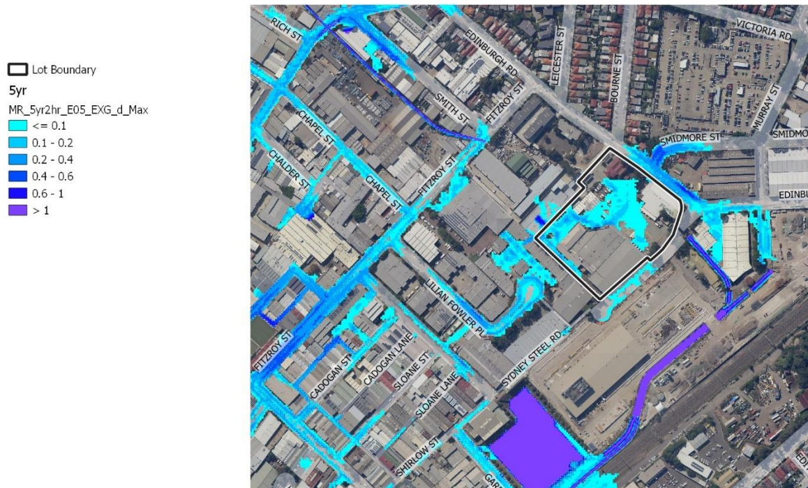
Figure 11 Pre Development 20% AEP Flood Depth (m)
