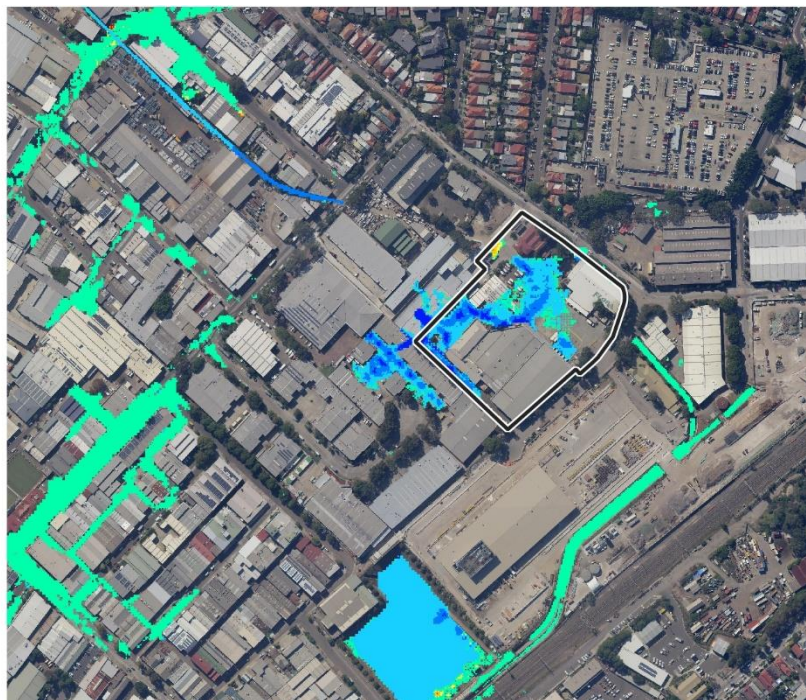
Figure 40 Post Development change in 5% AEP flood depth (m)
