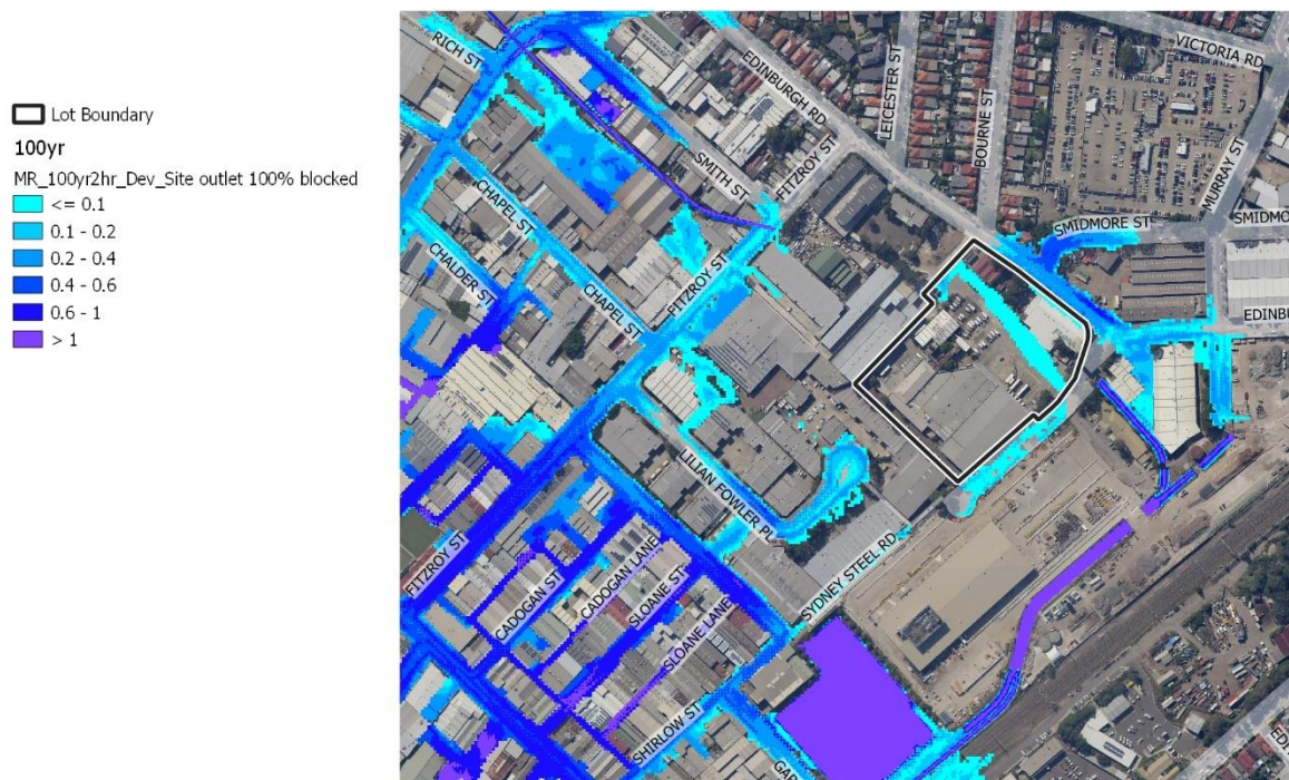
Figure 33 Post Development 1% AEP Flood Depth – Site outlet 100% blocked (m)
