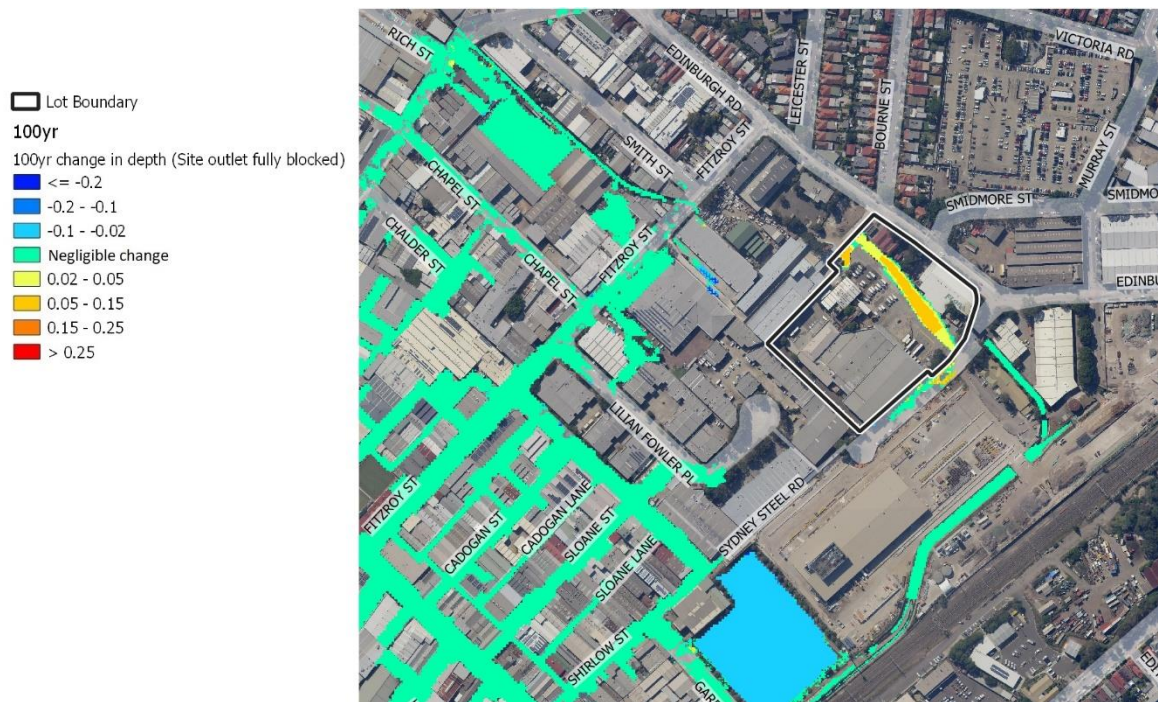
Figure 43 Post Development change in 1% AEP flood depth – Site outlet 100% blocked (m)
