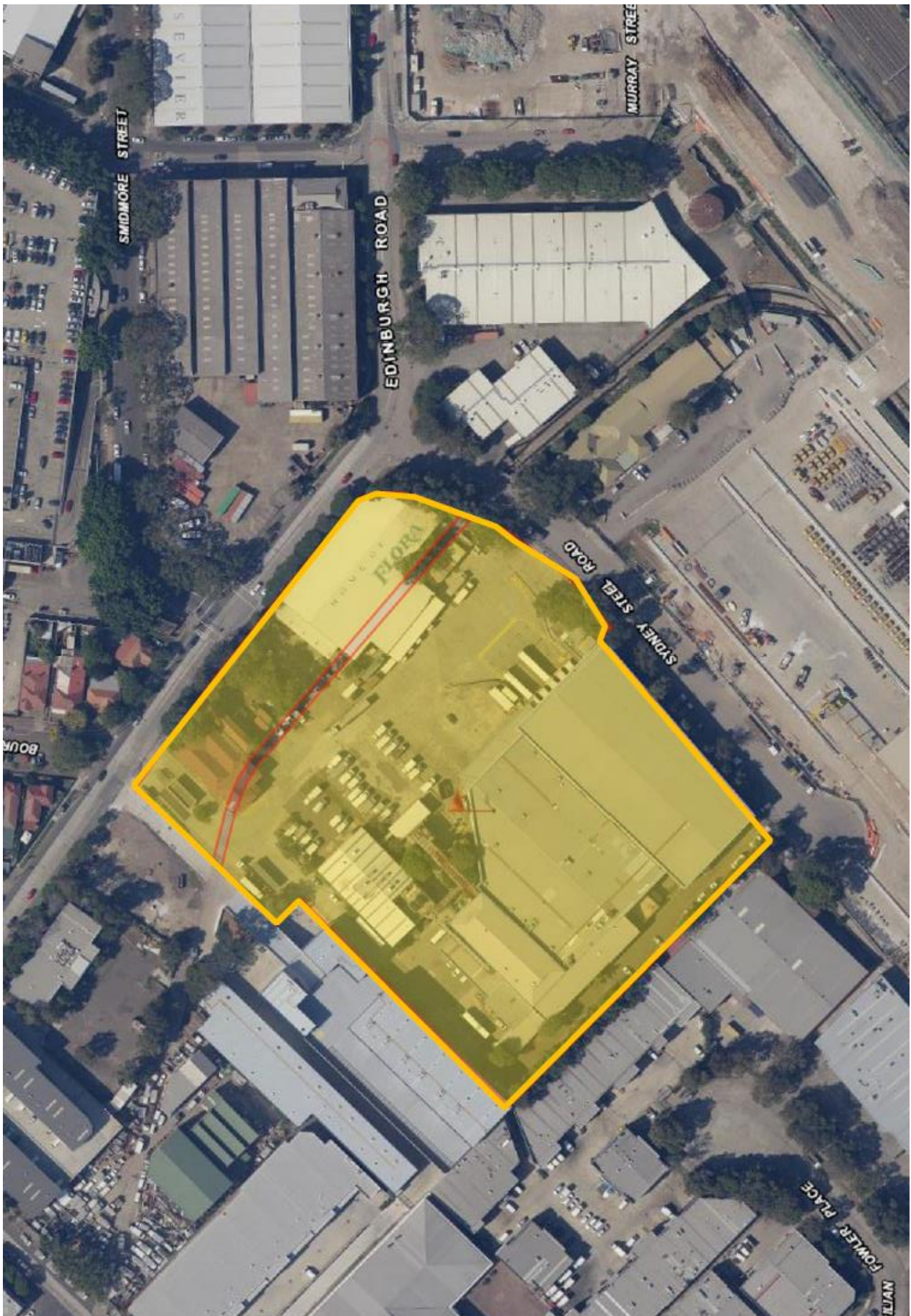
Figure 1 – Aerial view of the Site/subject area (yellow polygon) with the approximate alignment subsurface canal in red. Source: Six Maps
