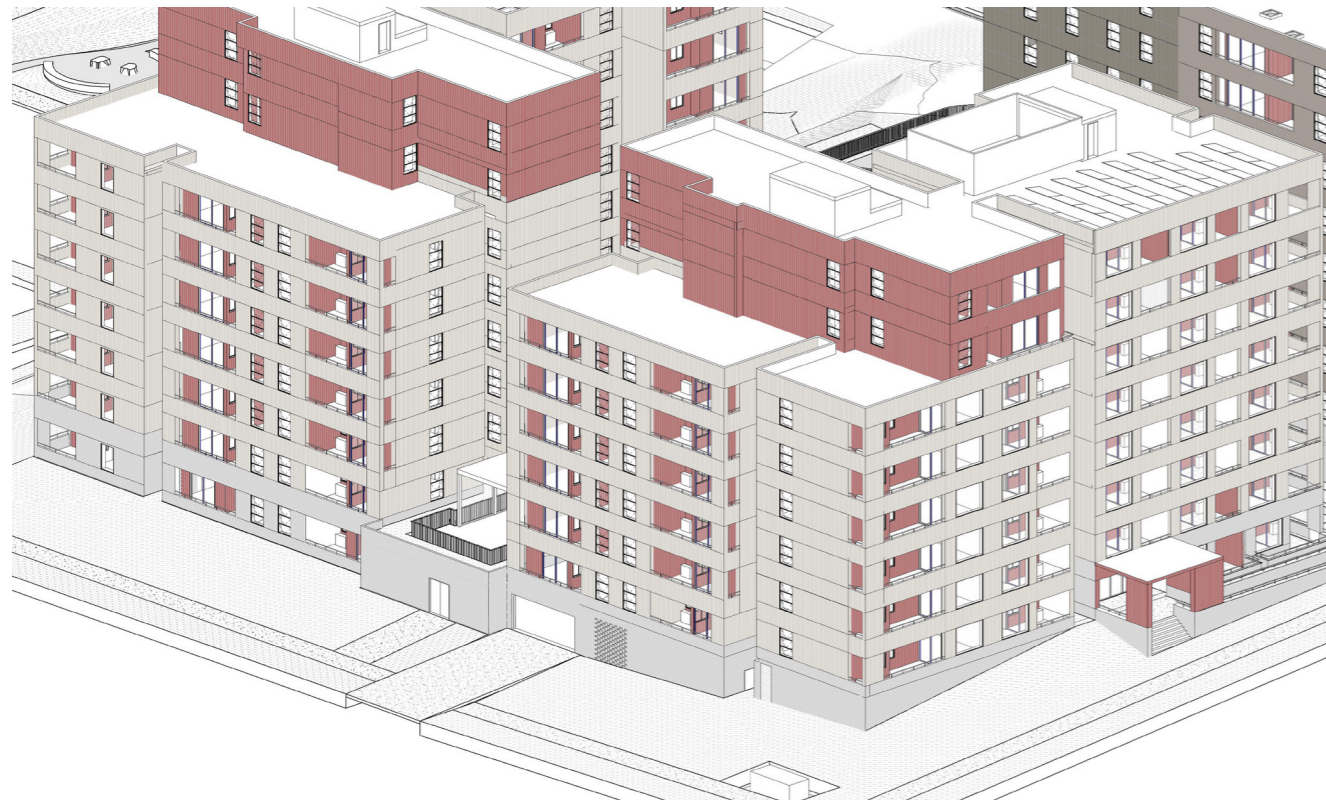
AXONOMETRIX VIEW OF SOCIAL HOUSING BUILDING SHOWING LEVEL DIFFERENCE FOR LOWER LEVEL RESIDENTIAL APARTMENTS WTIHOUT PRIVATE OPEN SPACE TO NATURAL GROUND
