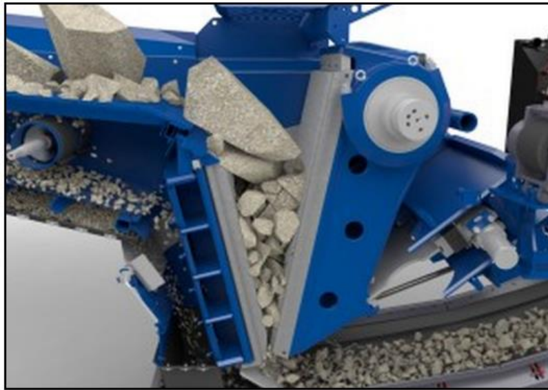
Figure 2-4 Typical Jaw Crusher Operation
