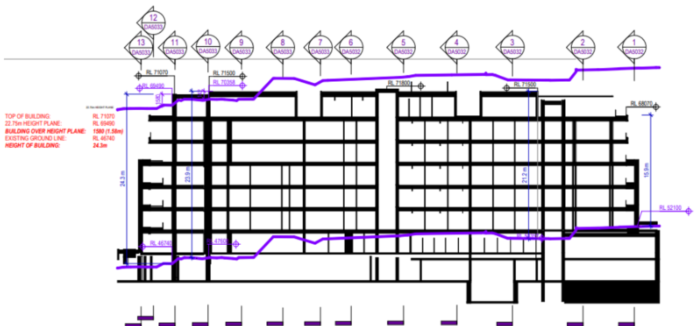
Figure 12 Long section showing height exceedance above the 22.75m height plane
