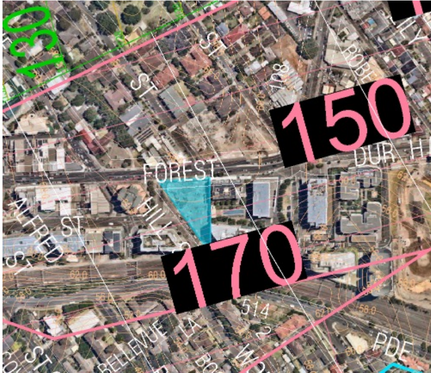
Diagram 1: Height of PANS-OPS Surface at 1a Hill St and 105 Forest Rd
