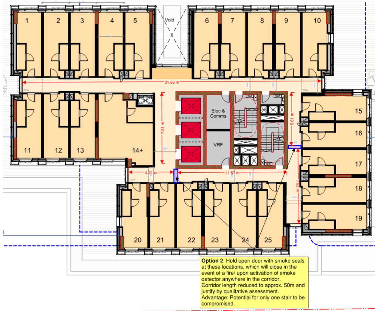
Figure 3: Option 2: Hold Open Door with Smoke seals
