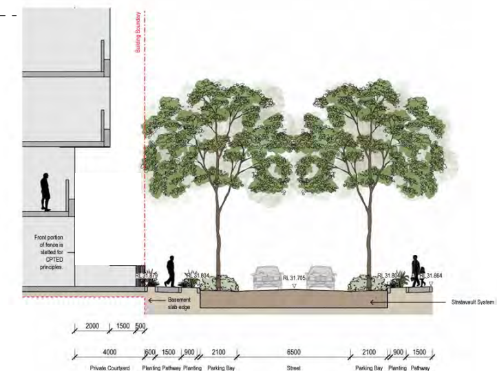
4 INTERNAL STREET SECTION
