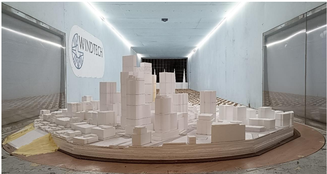
Figure 1e: Photograph of the Wind Tunnel Model (view from the north-west)
