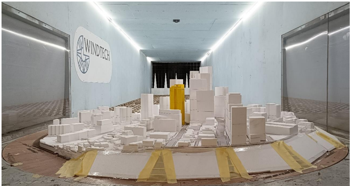
Figure 1c: Photograph of the Wind Tunnel Model (view from the south-east)
