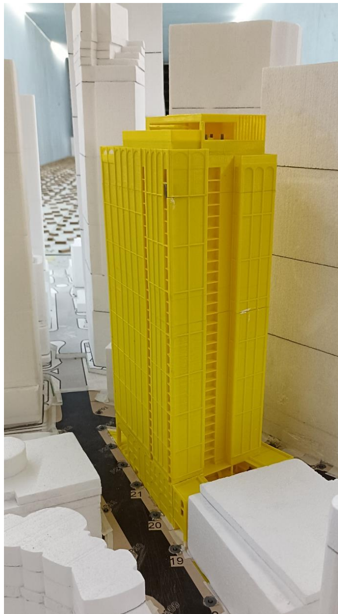
Figure 1a: Photograph of the Wind Tunnel Model (view from the south)
