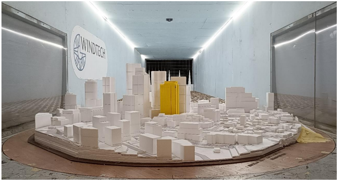
Figure 1d: Photograph of the Wind Tunnel Model (view from the south-west)
