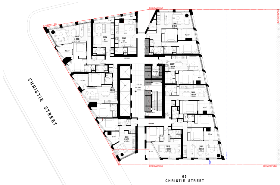
Typical floor plan of the Telstra Exchange BTR development (south-west elevation to the south of this image)
