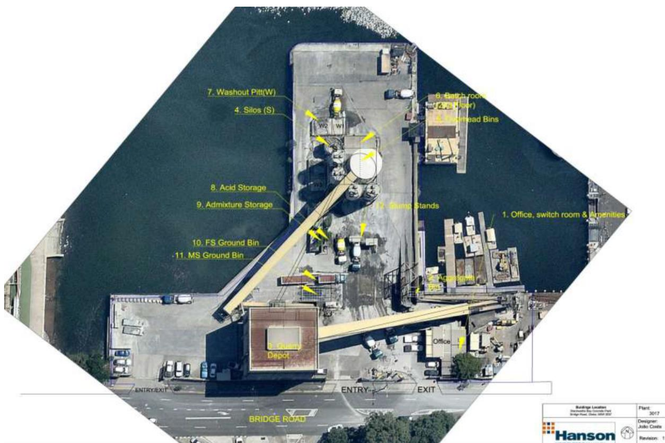
Figure 2 – Existing Structures to be demolished
