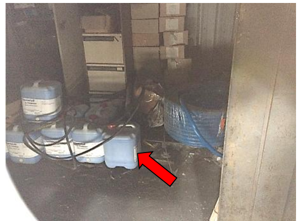
Photo 21: Cleaning chemicals stored without secondary containment within a locked area on the eastern side of the tanker route
