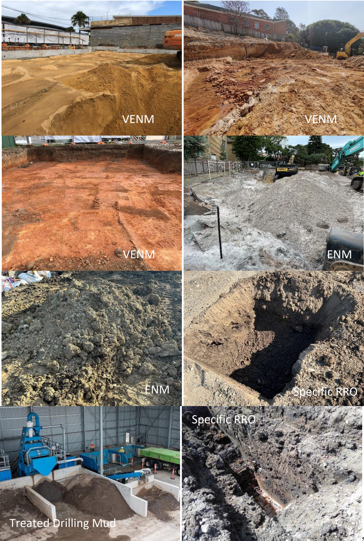
Figure 5: Example images of recycled soil materials classified under fill and earthworks RRO/RRE's. Materials as labelled.
