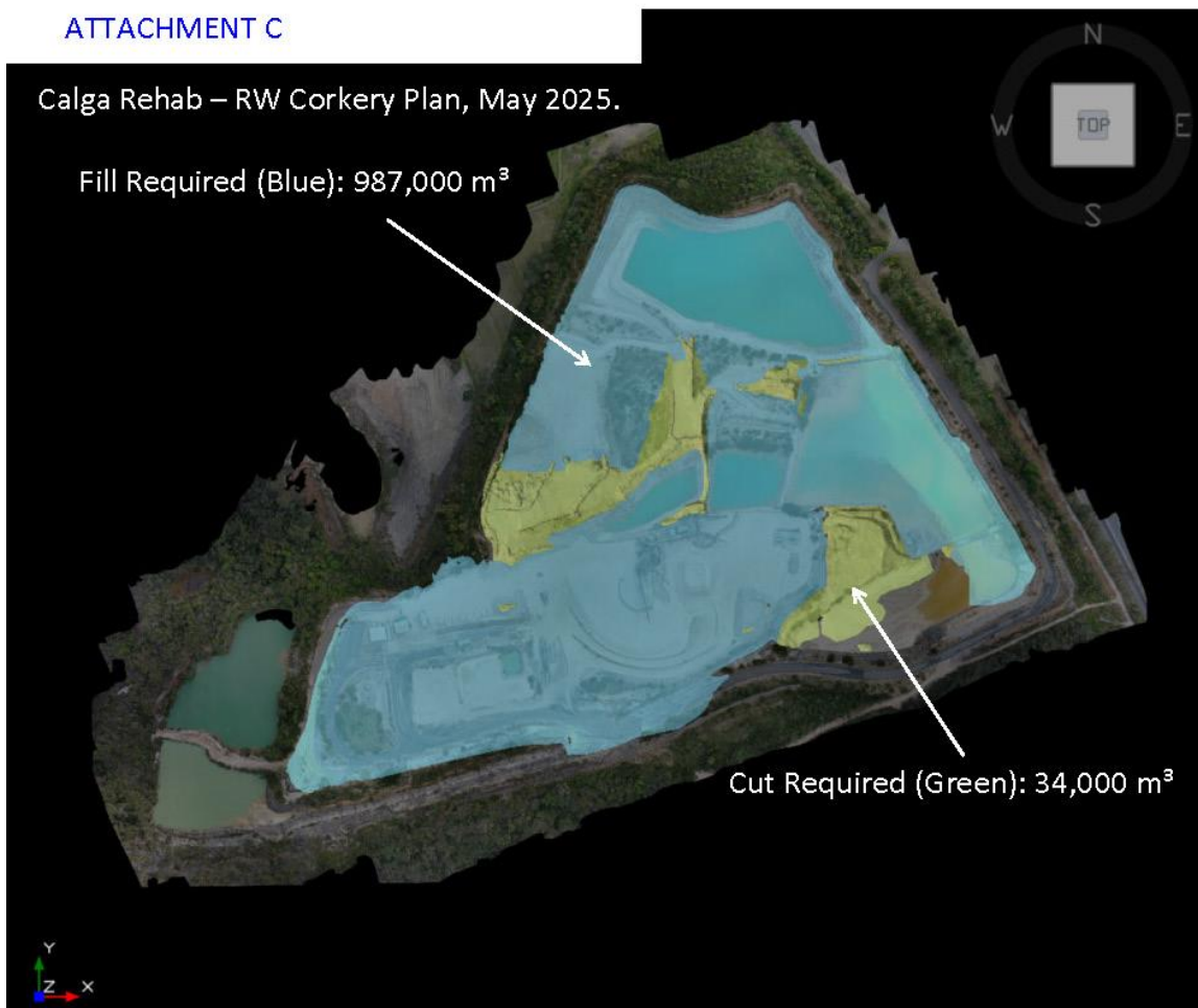
Figure 9: Cut and fill diagram for the pit - excerpt from 2025 updated Rehabilitation and Landscape Management Plan, prepared by RW Corkery and Co.
