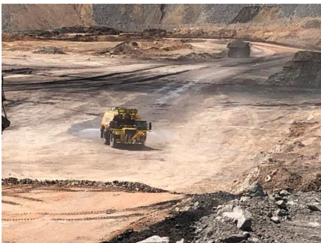
Photo Air 4 - Water trucks being effectively used on 26 February 2020 along the haulage route
