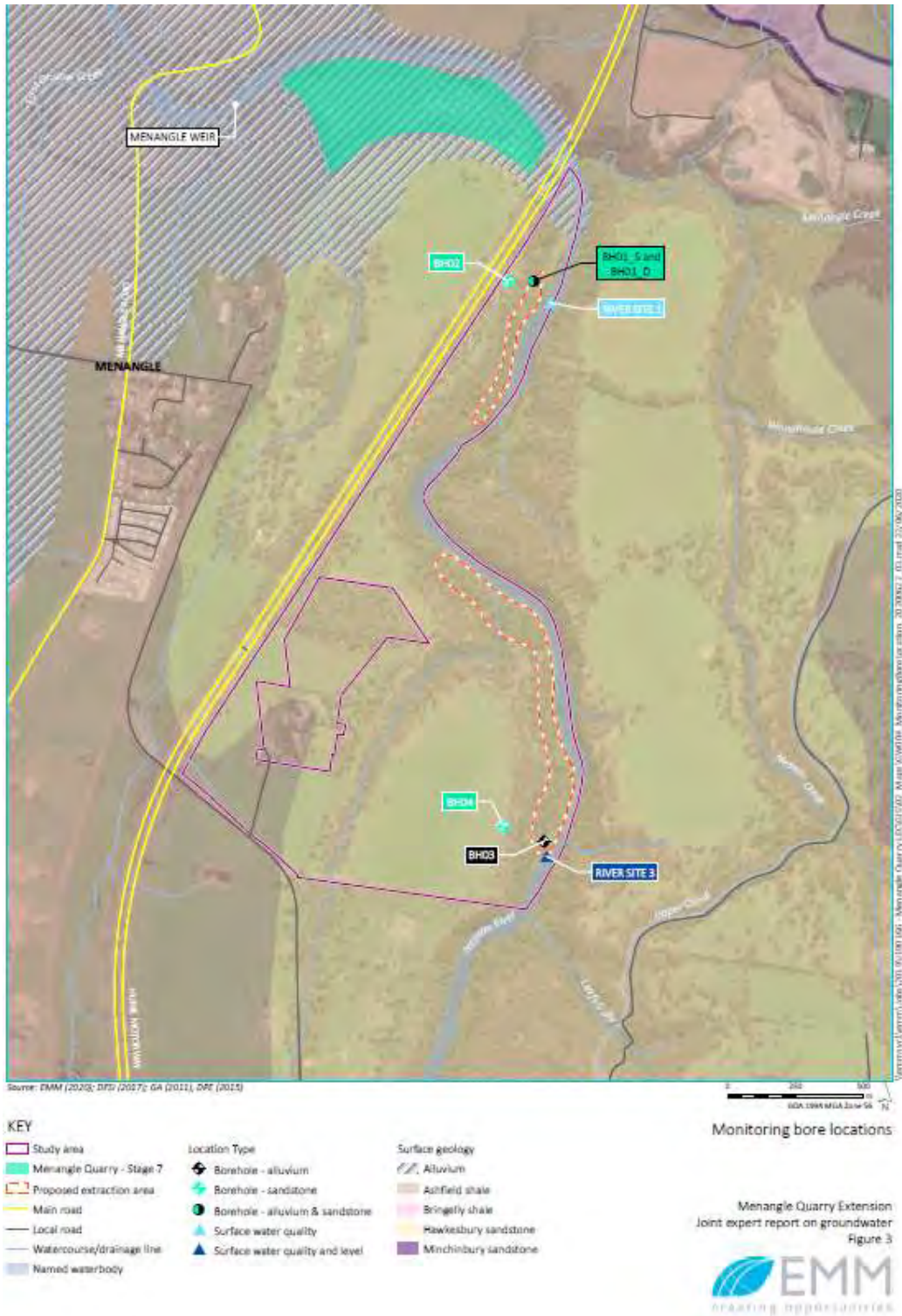
Figure 7 - Groundwater Monitoring Locations
