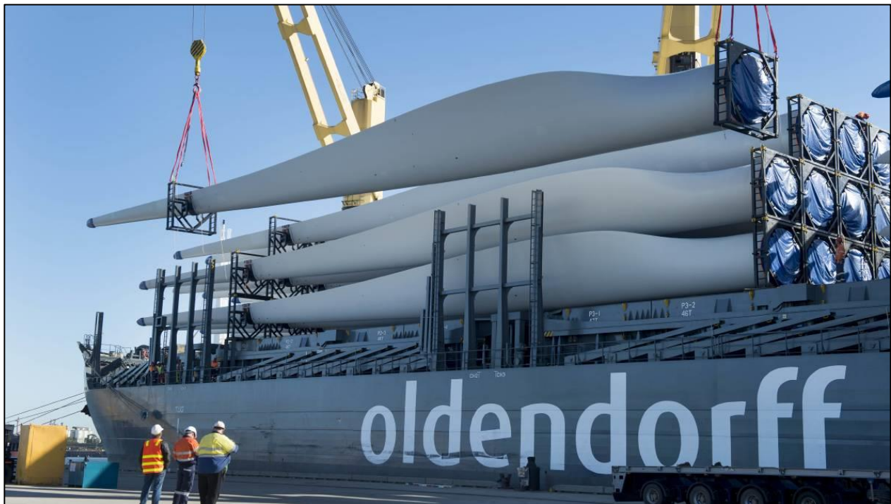
Figure 6: Wind turbine blades being unloaded using ship's cranes, as proposed.
