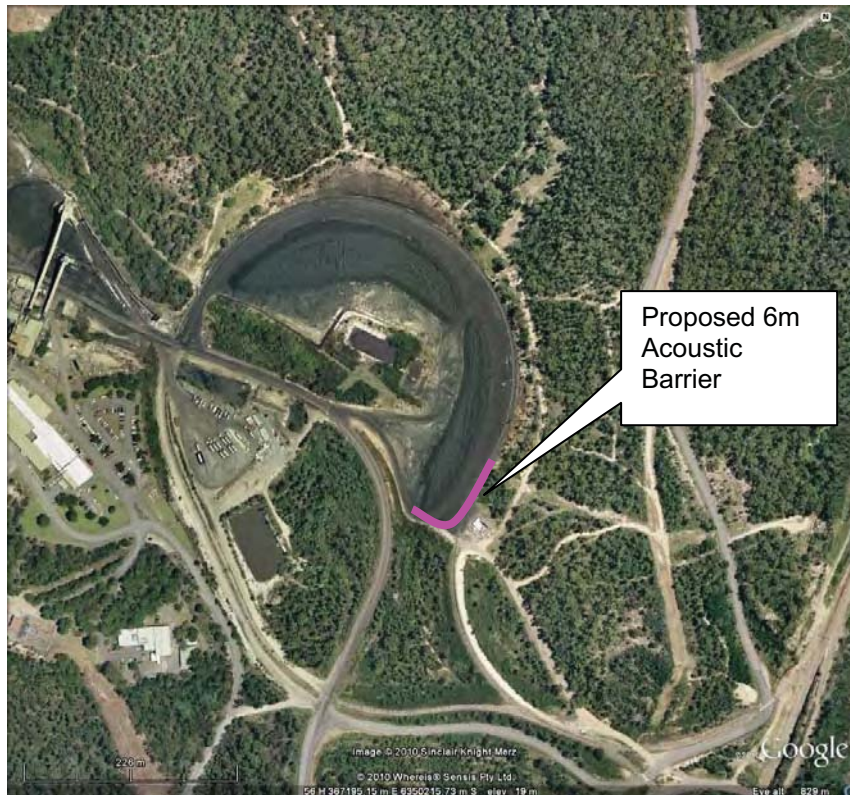
Figure 5 Proposed 6m noise bund – Coal Train Rail Loop
