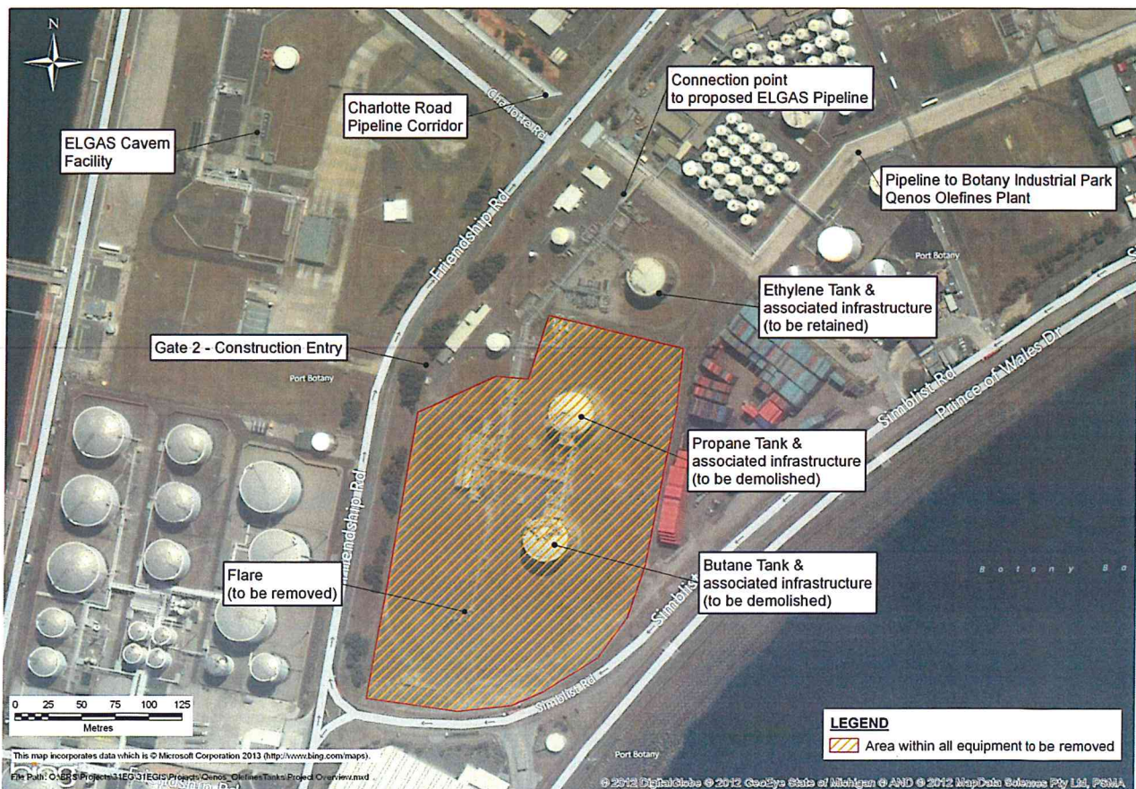
Figure 3: Site infrastructure including the tanks to be demolished.
