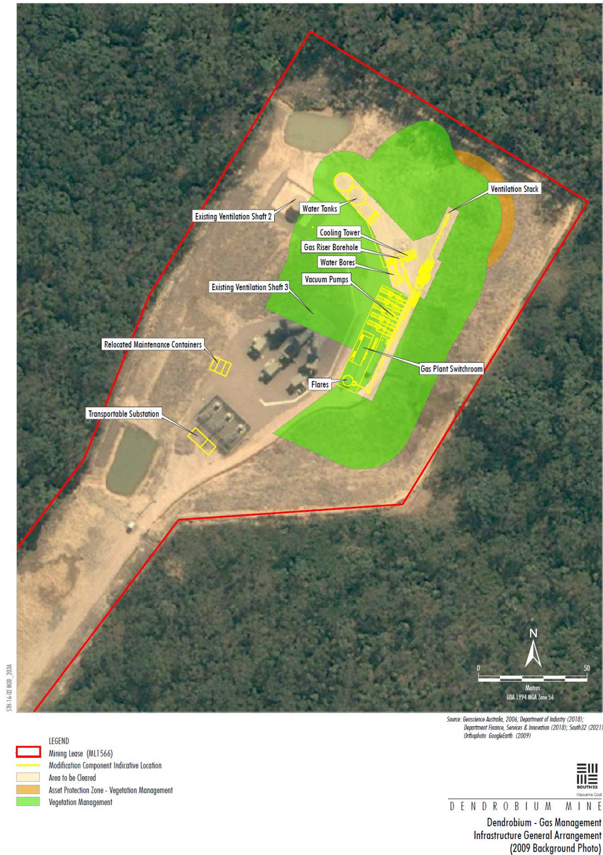
Figure 2 Gas Management Infrastructure General Arrangement
