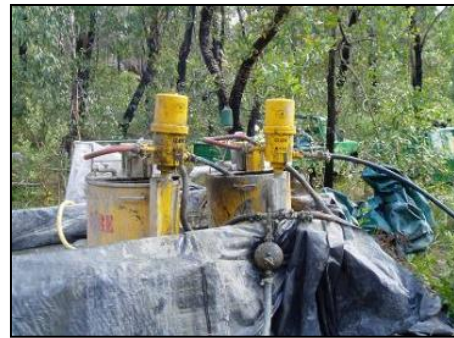
(b) Grout pump station setup
