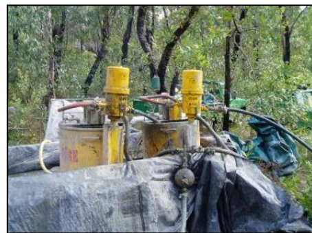
(b) Grout pump station setup
