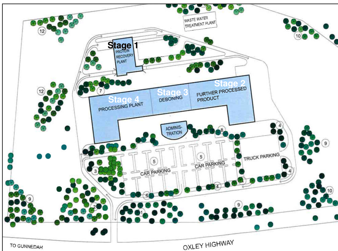
Figure 3 – Original 1998 site layout and facilities
