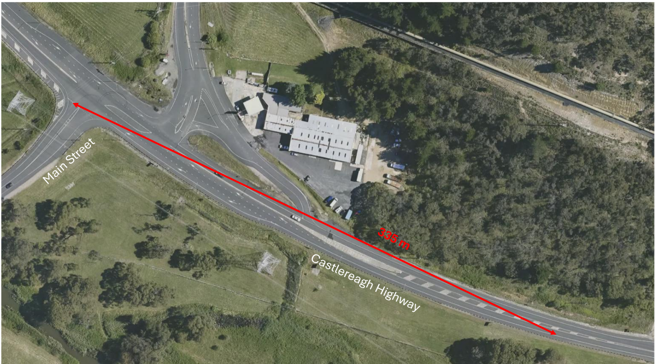
Figure 4.6 Sight distance to the right from Main Street to Castlereagh Highway (335 m)
