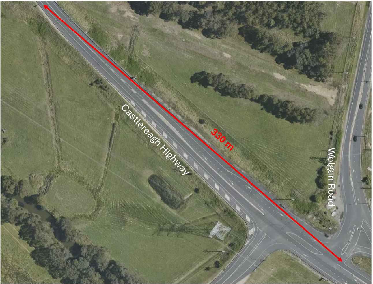
Figure 4.8 Sight distance to the right from Wolgan Road to Castlereagh Highway (330 m)
