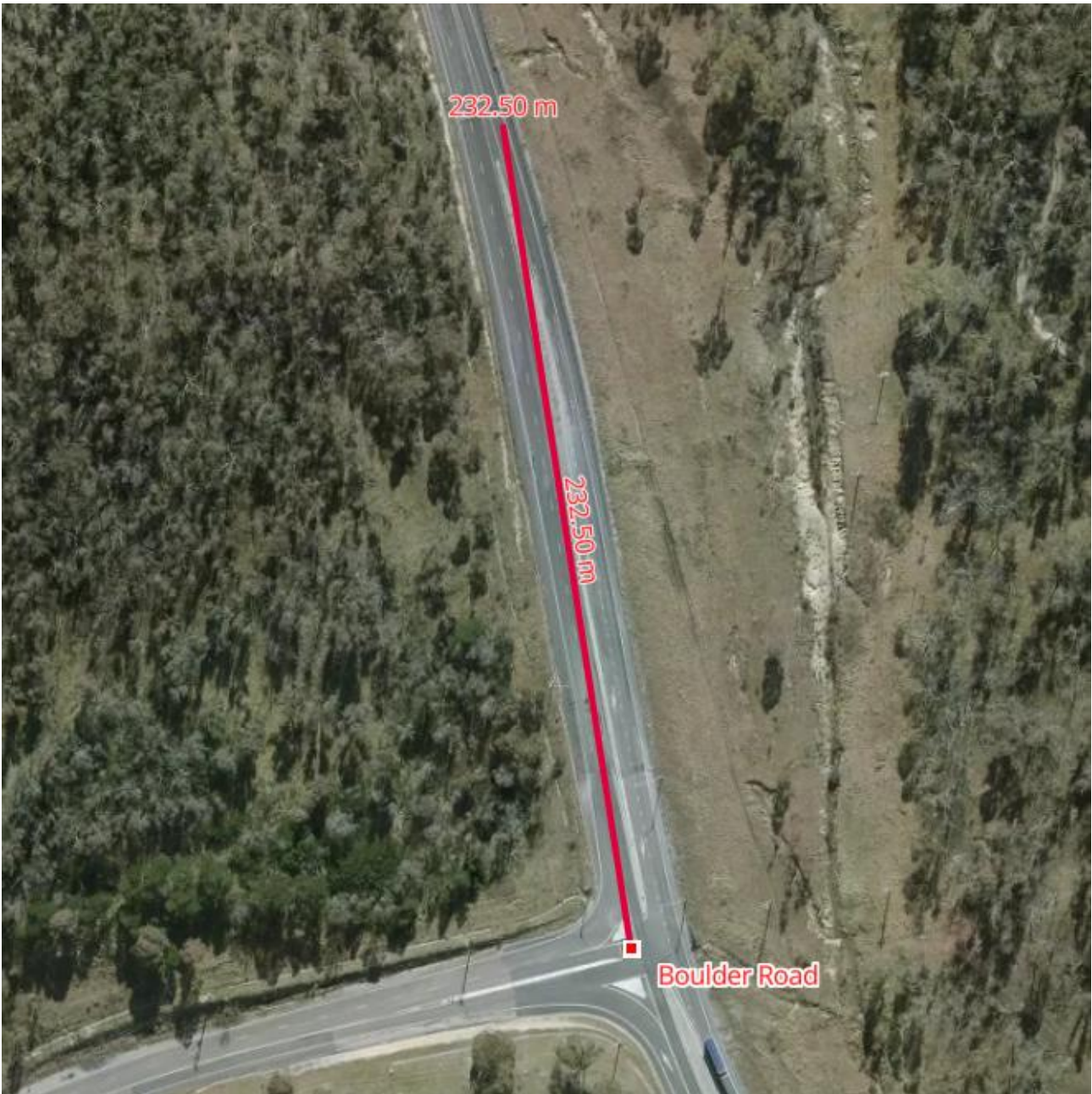
Figure 4.9 Sight distance to the left from Boulder Road to Castlereagh Highway (232 m)
