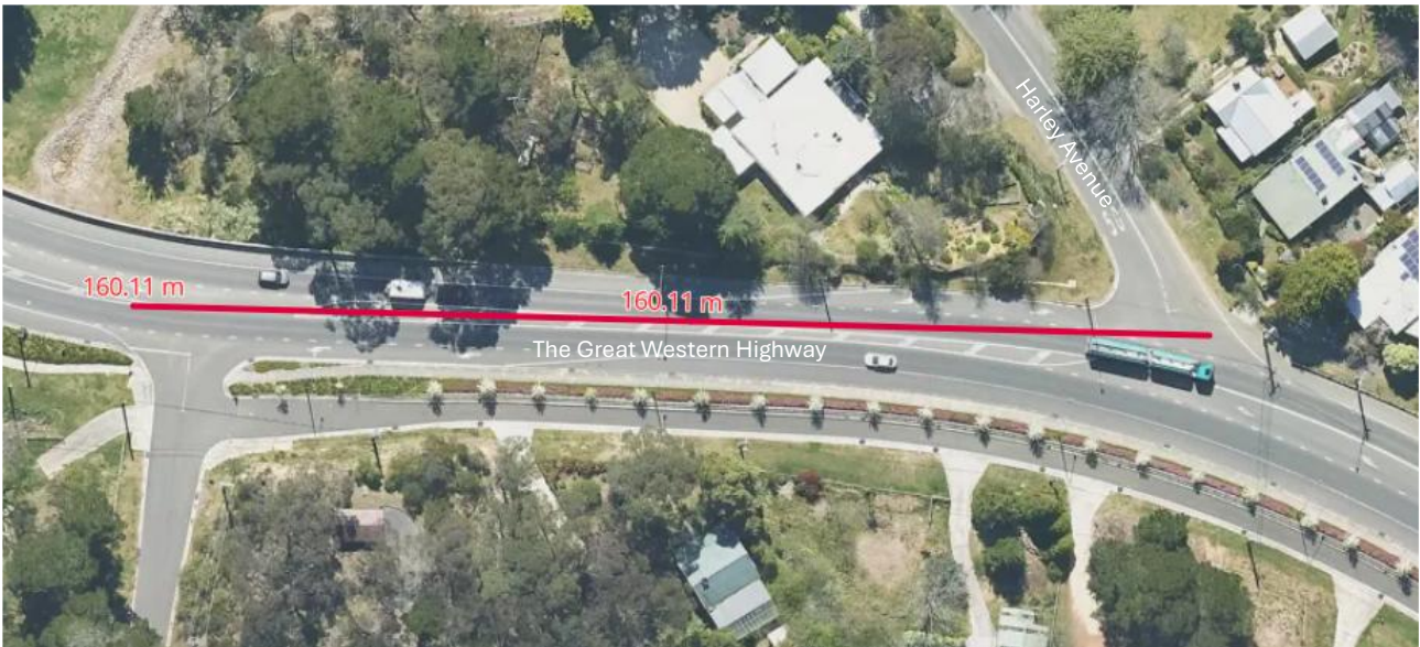
Figure 4.4 Sight distance to the right from Harley Avenue to Great Western Highway (160 m)
