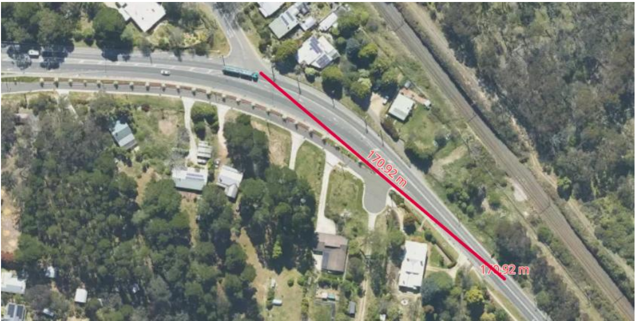
Figure 4.3 Sight distance to the left from Harley Avenue to Great Western Highway (170 m)
