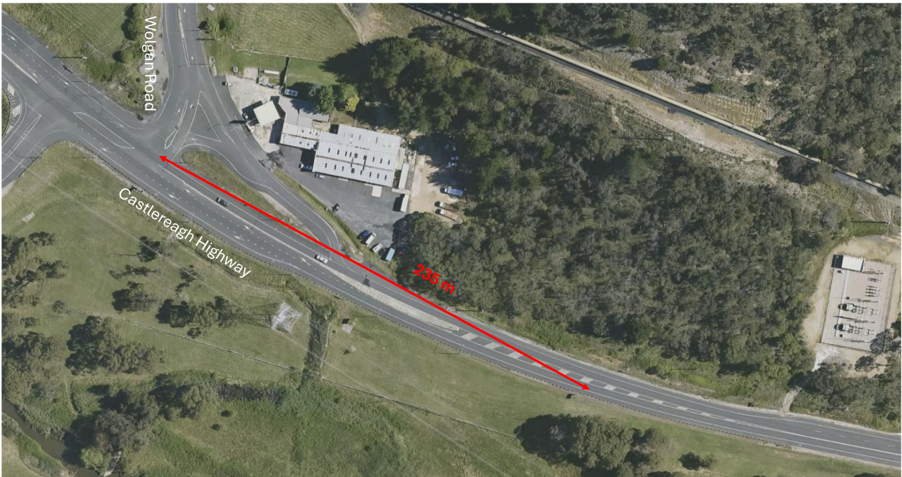
Figure 4.7 Sight distance to the left from Wolgan Road to Castlereagh Highway (235 m)
