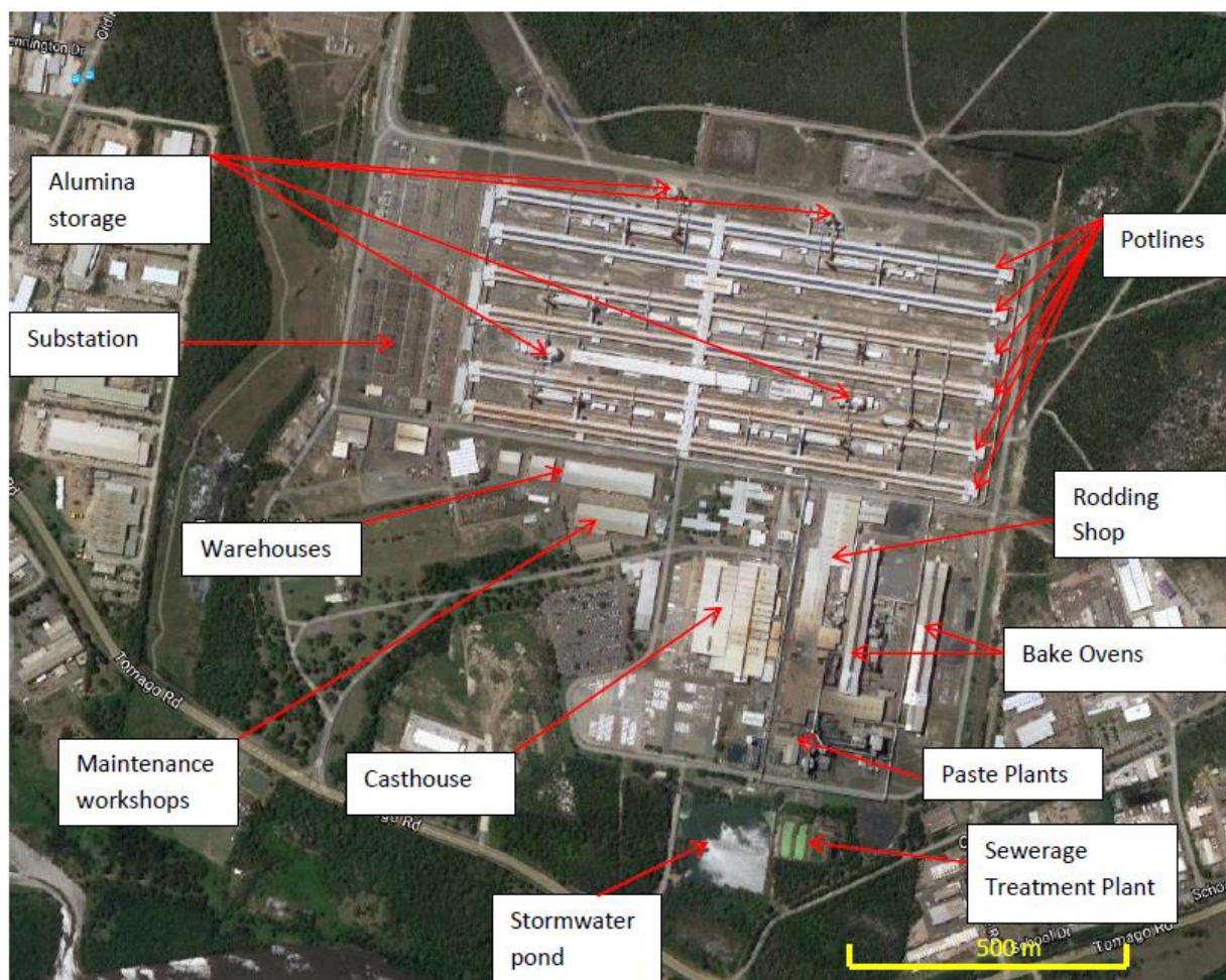
Figure 2.4: Site facilities and infrastructure
