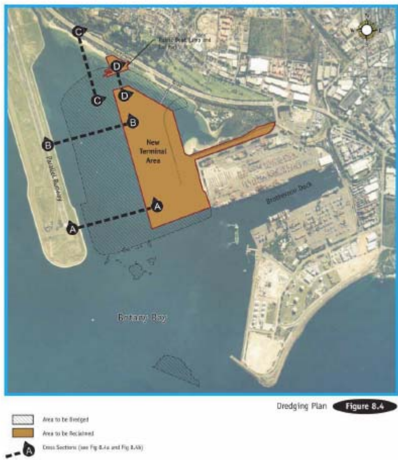
Figure 1: Approved Dredging and Reclamation (From URS, 2003)
