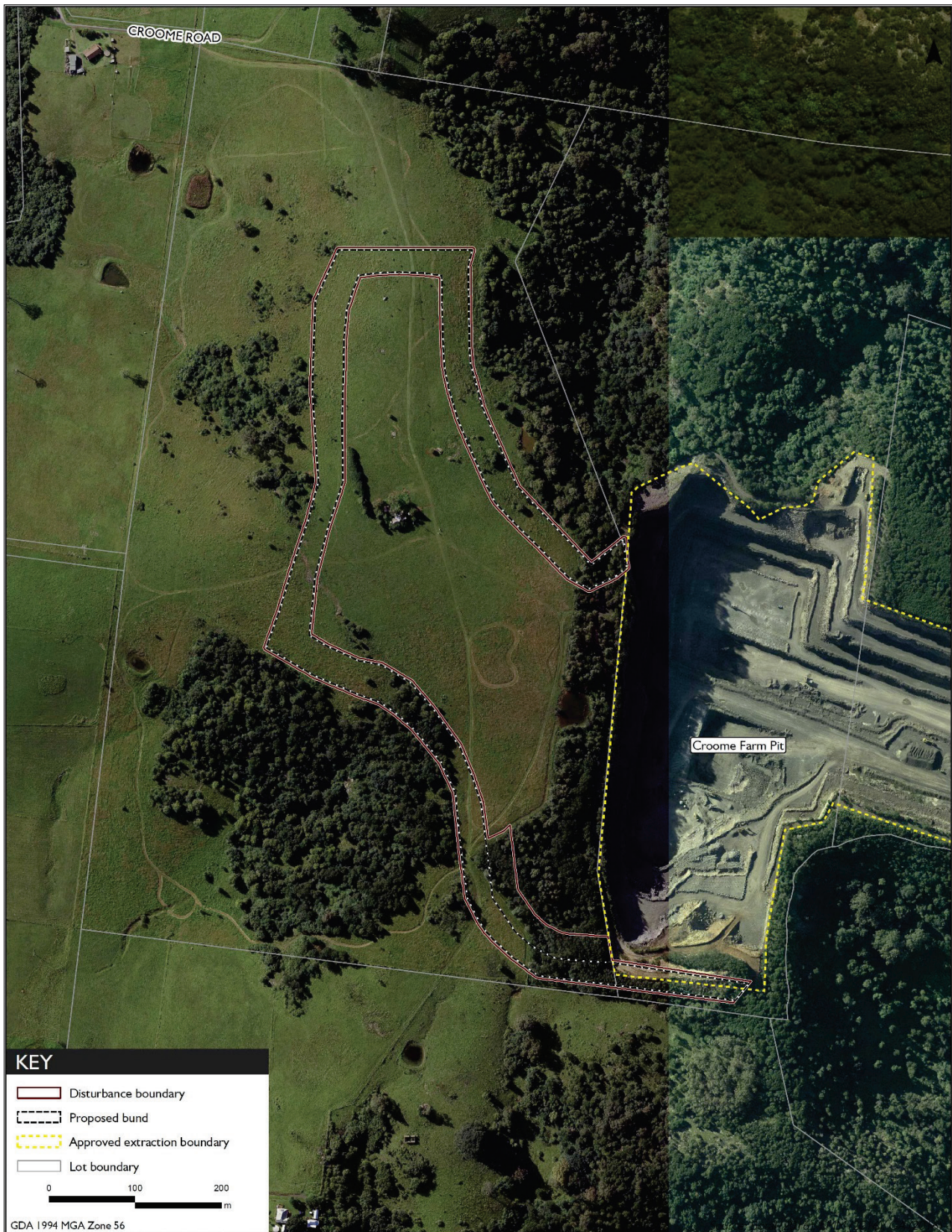
Figure 1-1: Proposed bund construction area
