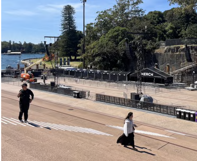
Figure 35:: View to black clad BAR and MERCH tents arranged in a single row in proximity to the Tarpein Wall. Temporary self-adhesive nosing strips are added to the Monumental Steps for events and then later removed. Testing has been undertaken to ensure that the adhesive does not dislodge granite chips when removed.
