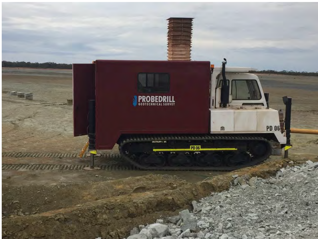
Plate 3 - CPT Testing Rig
