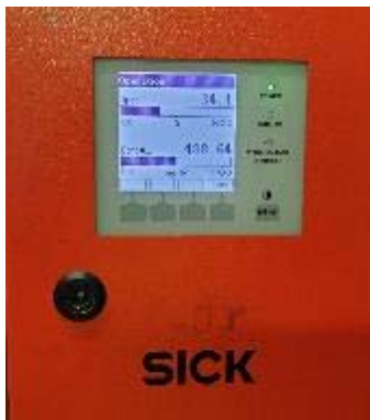
Photo 4: Boiler emissions opacity monitor reading 30-50%; minimal smoke evidence at 34.1%.
