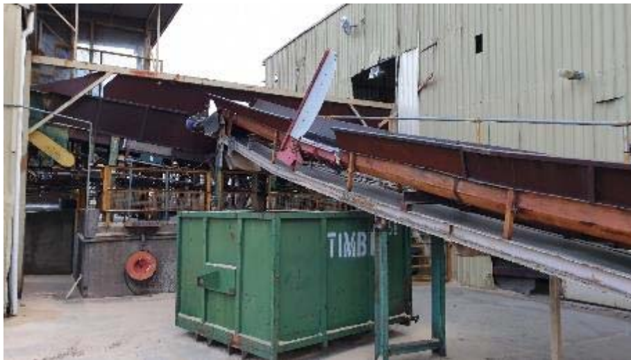
Photo 2a: Docking of Holtec treated timbers can feed into timber bin destined for chipping and boiler fuel.
