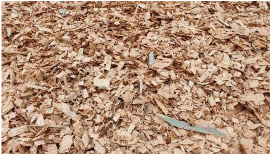
Photo 1: Chip contains small amounts of treated timber content (Blue frame pieces). Destined for boiler fuel.
