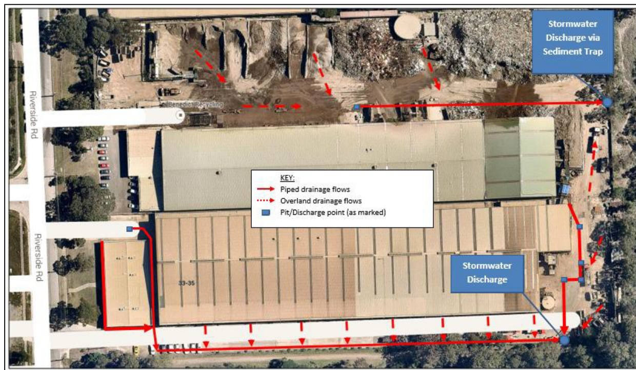
Figure OP 8 - Surface Stormwater Directional Flow
