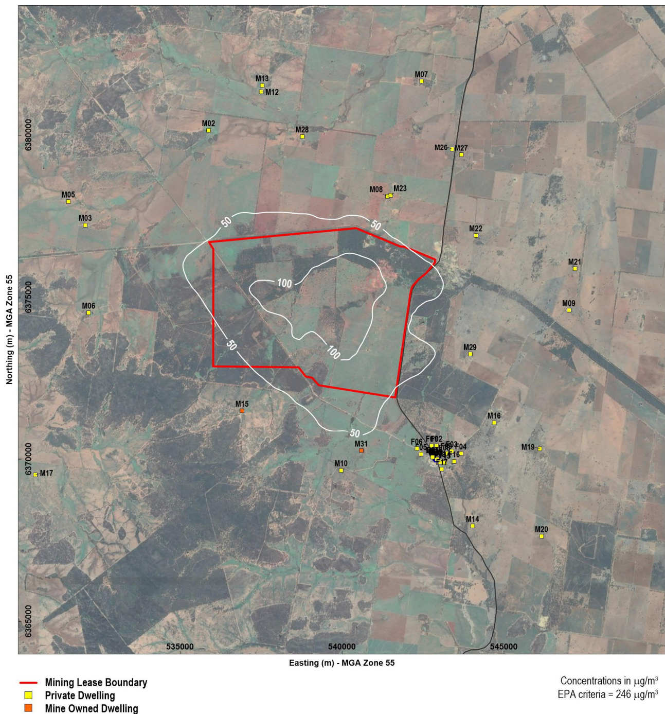
Figure 6.15 Modelled maximum 1-hour average \text{NO}_2 due to diesel exhausts
