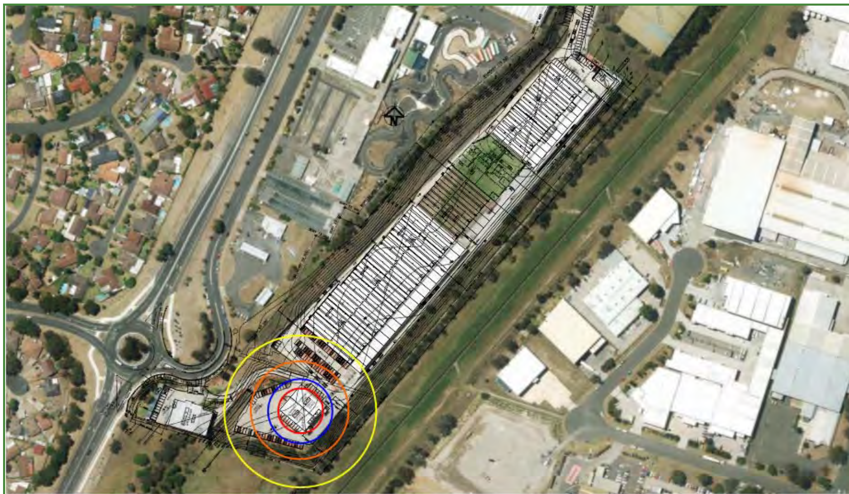
Figure 4-5: Heat Radiation Contours for Scenario 3: Bund fire involving 600,000 kg of Class 3 flammable liquids
