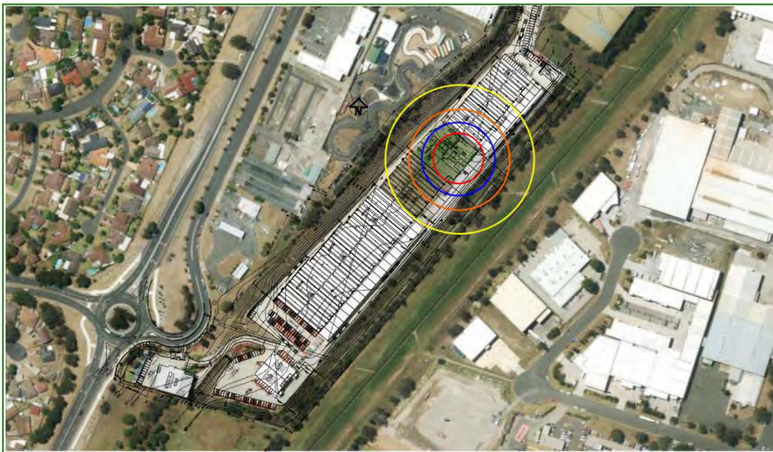
Figure 5-11: Heat Radiation Contours for Scenario 6: Fire involving 10,000 kg of Class 8(3) liquids
