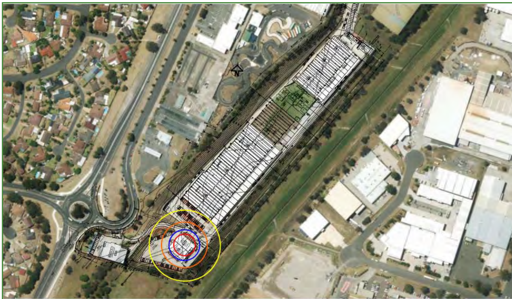
Figure 4-2: Heat Radiation Contours for Scenario 1: Pool fire involving 5,000 kg of Class 3 flammable liquids in B2
