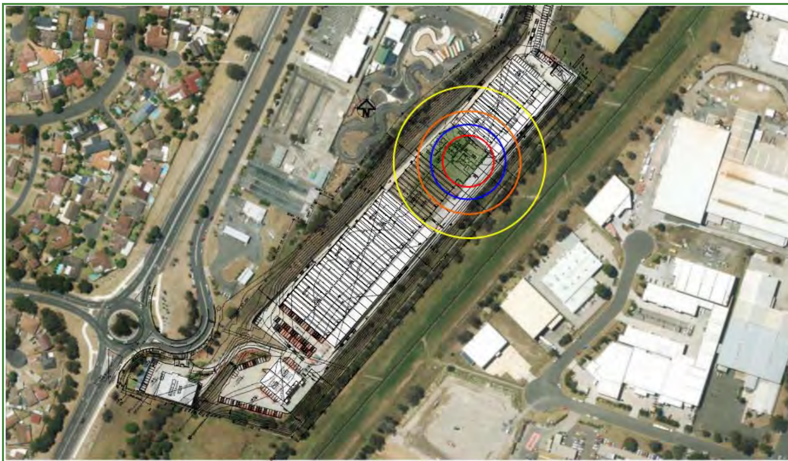
Figure 4-7: Heat Radiation Contours for Scenario 6: Fire involving 10,000 kg of Class 8(3) liquids
