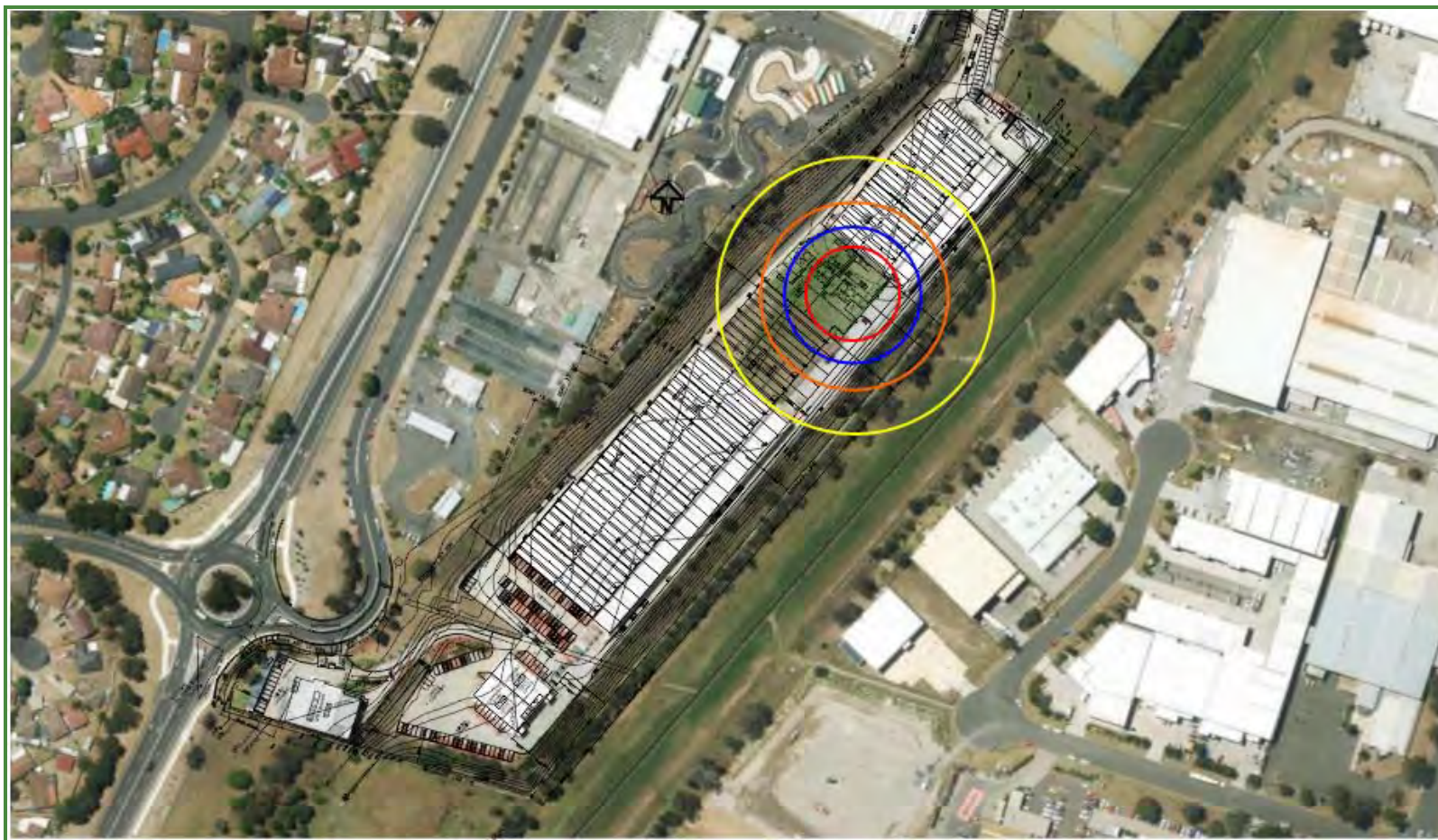
Figure 4-8: Heat Radiation Distances for Scenario 7: Fire involving 30,000 kg of Class 8(3) liquid
