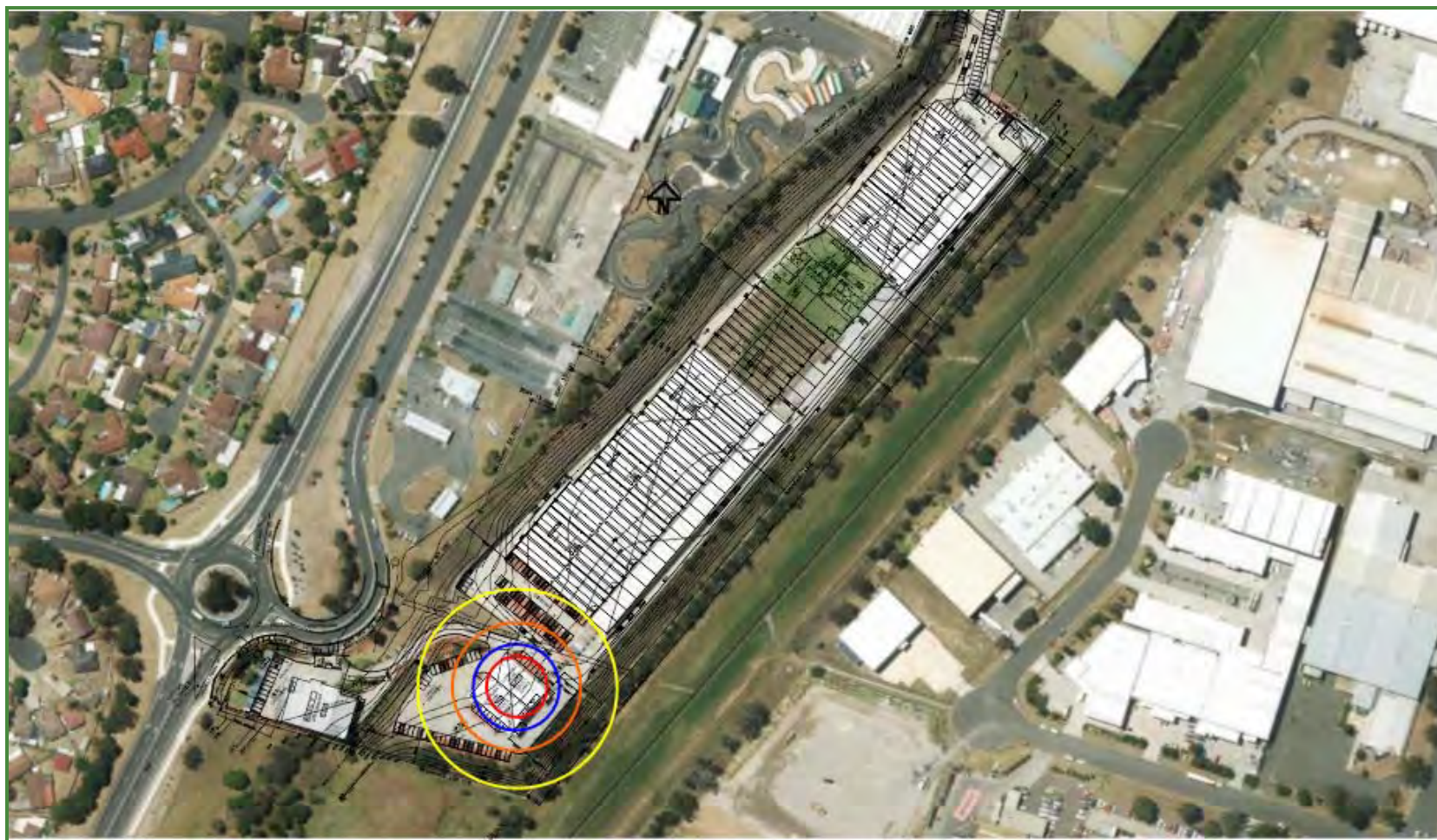
Figure 4-4: Heat Radiation Contours for Scenario 2: Pool fire involving 30,000 kg of Class 3 flammable liquids in B2
