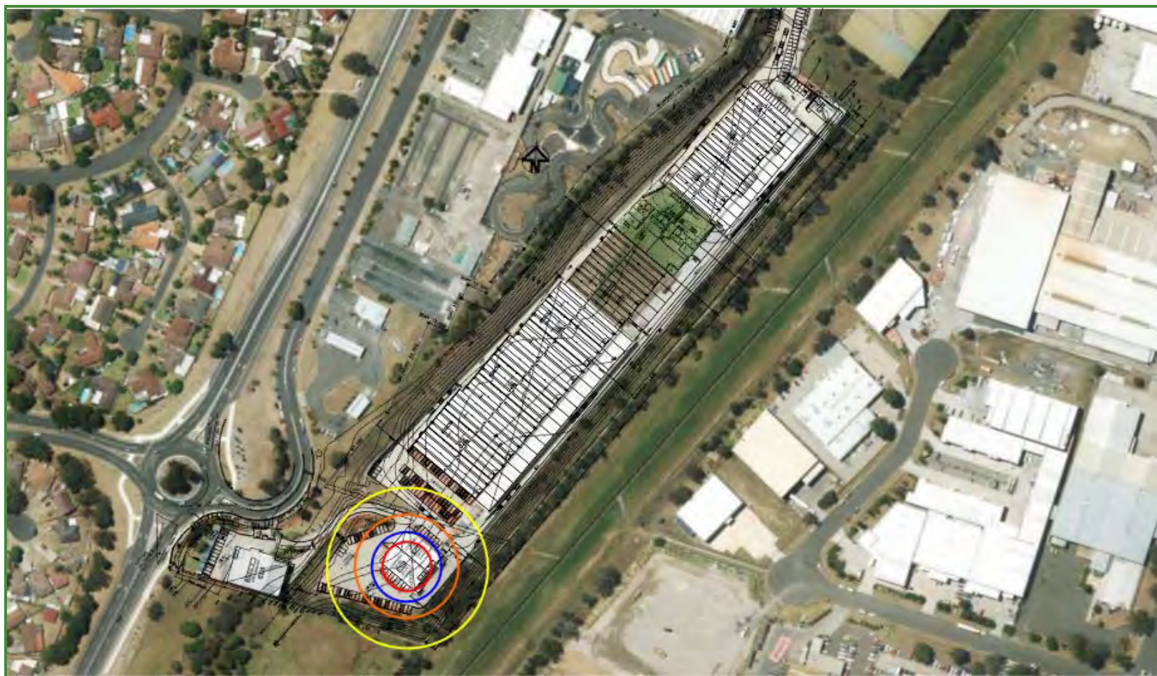
Figure 4-3: Heat Radiation Contours for Scenario 2: Pool fire involving 30,000 kg of Class 3 flammable liquids in B1
