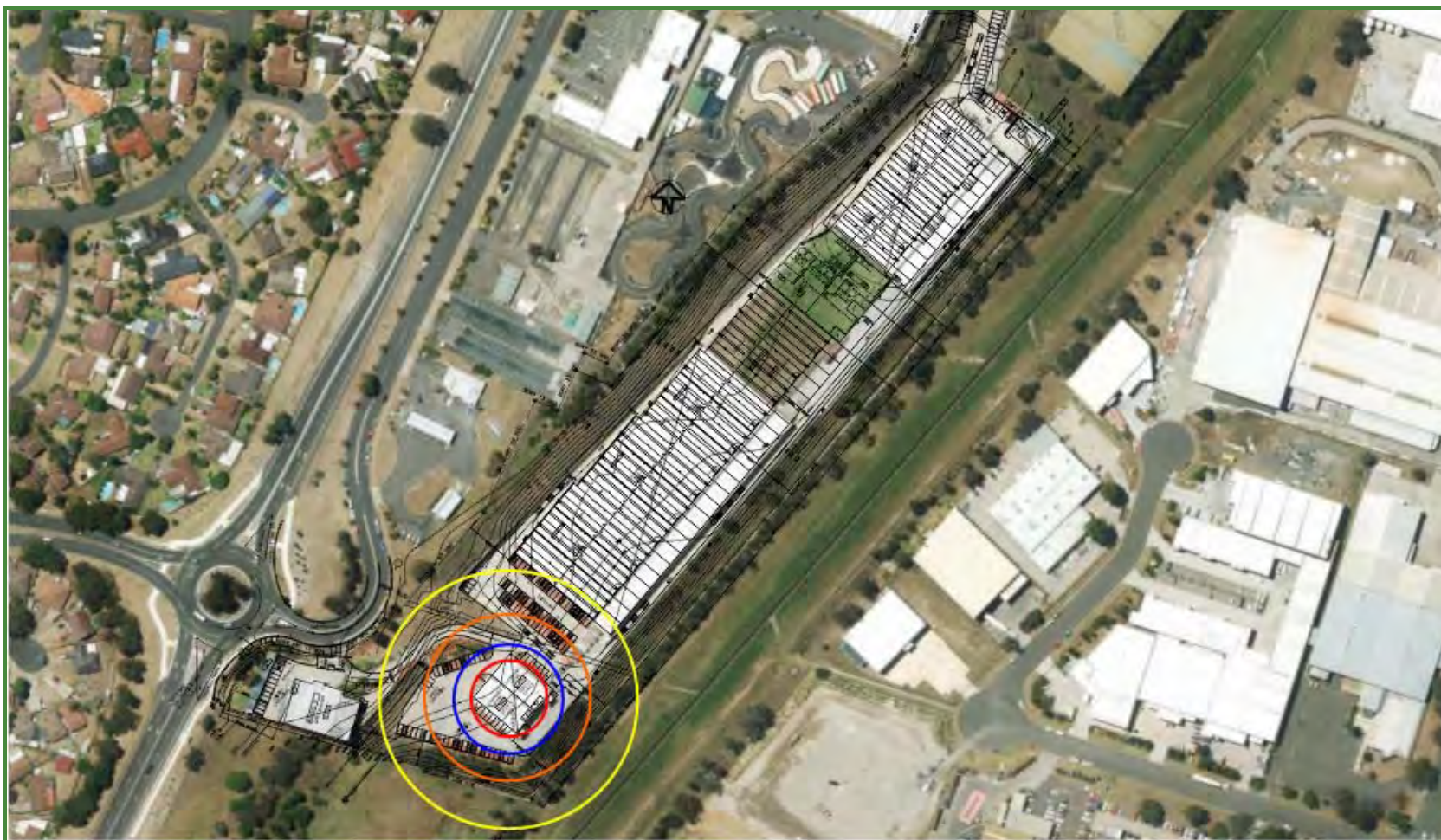
Figure 5-9: Heat Radiation Contours for Scenario 3: Bund fire involving 600,000 kg of Class 3 flammable liquids
