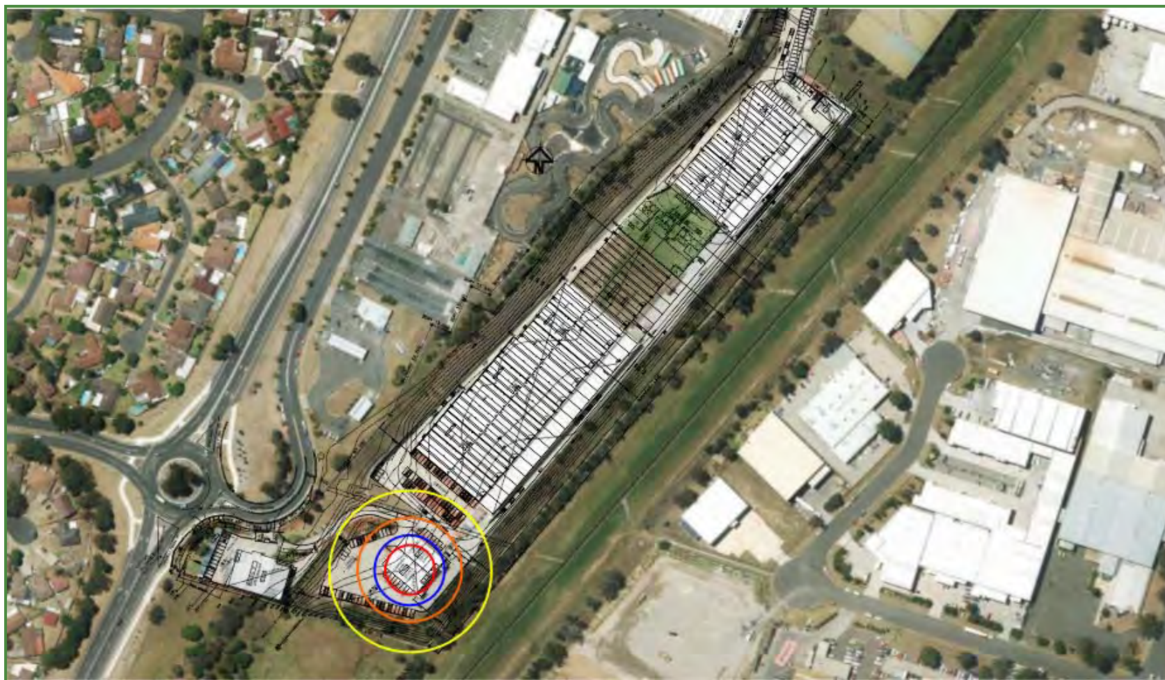
Figure 5-5: Heat Radiation Contours for Scenario 1: Pool fire involving 5,000 kg of Class 3 flammable liquids in B1
