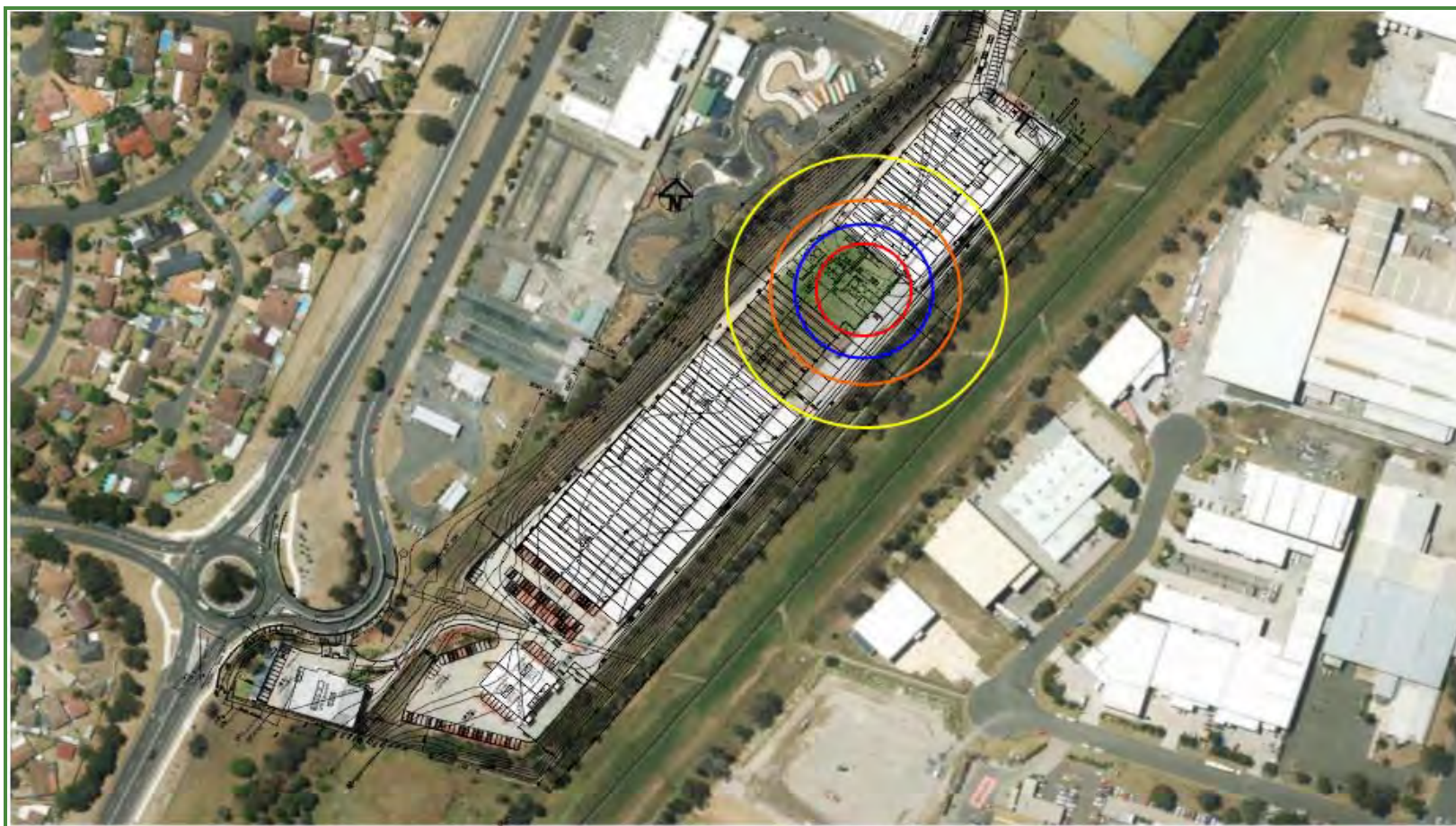
Figure 4-6: Heat Radiation Contours for Scenario 5: Fire involving 3,000 kg of Class 8(3) liquids
