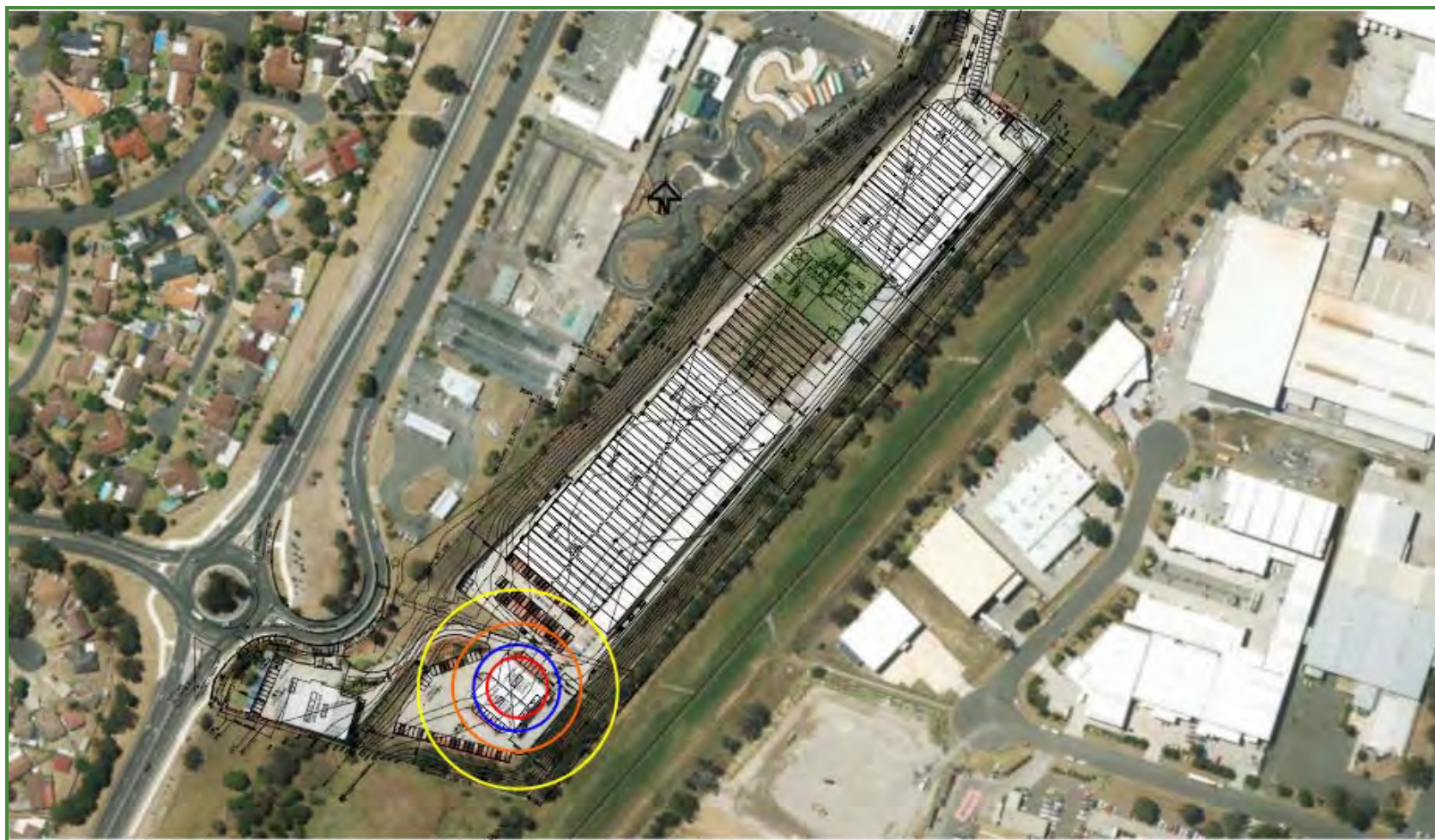
Figure 5-6: Heat Radiation Contours for Scenario 1: Pool fire involving 5,000 kg of Class 3 flammable liquids in B2
