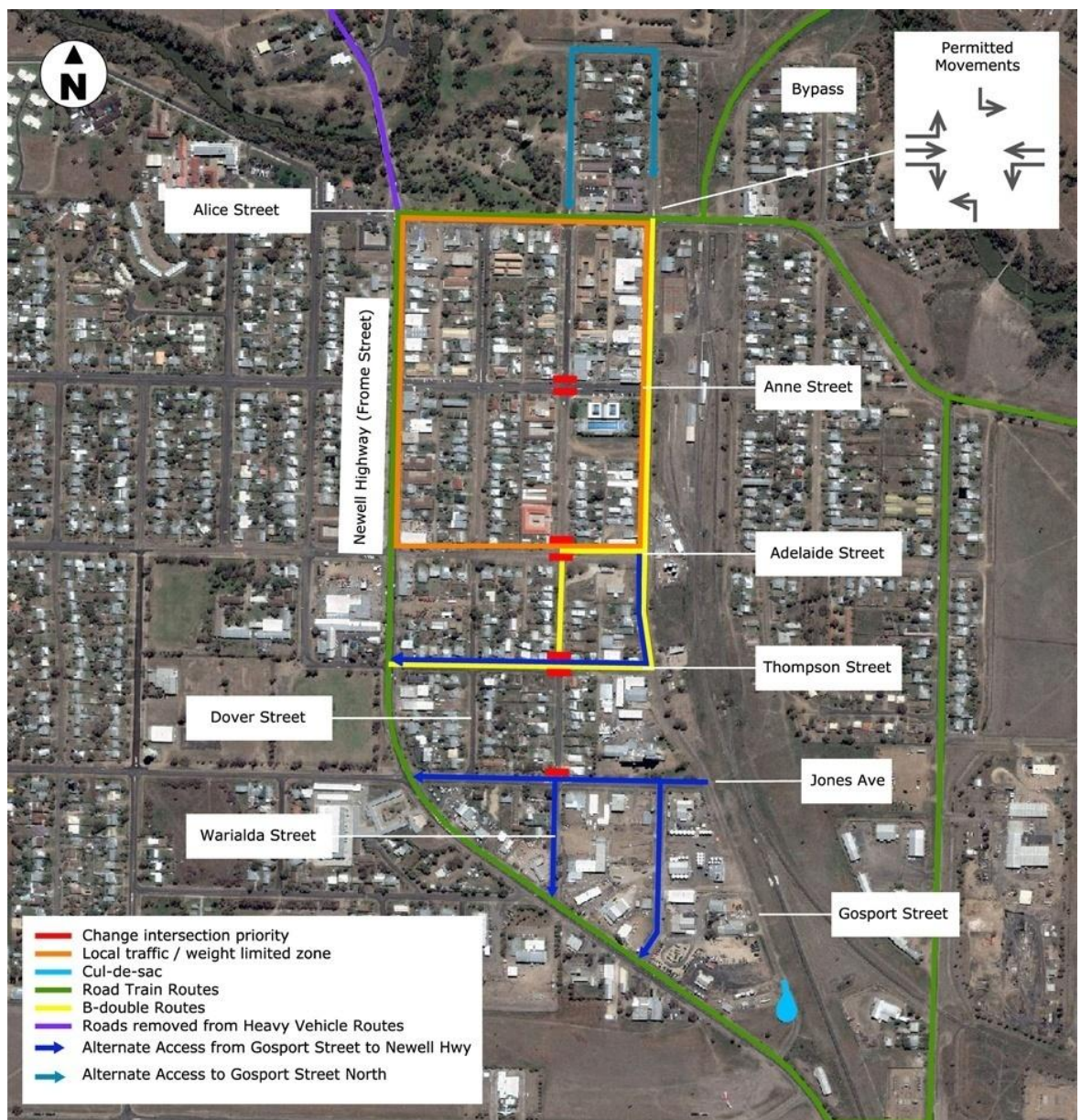
Figure 6-11: Phase 1 Traffic arrangements
