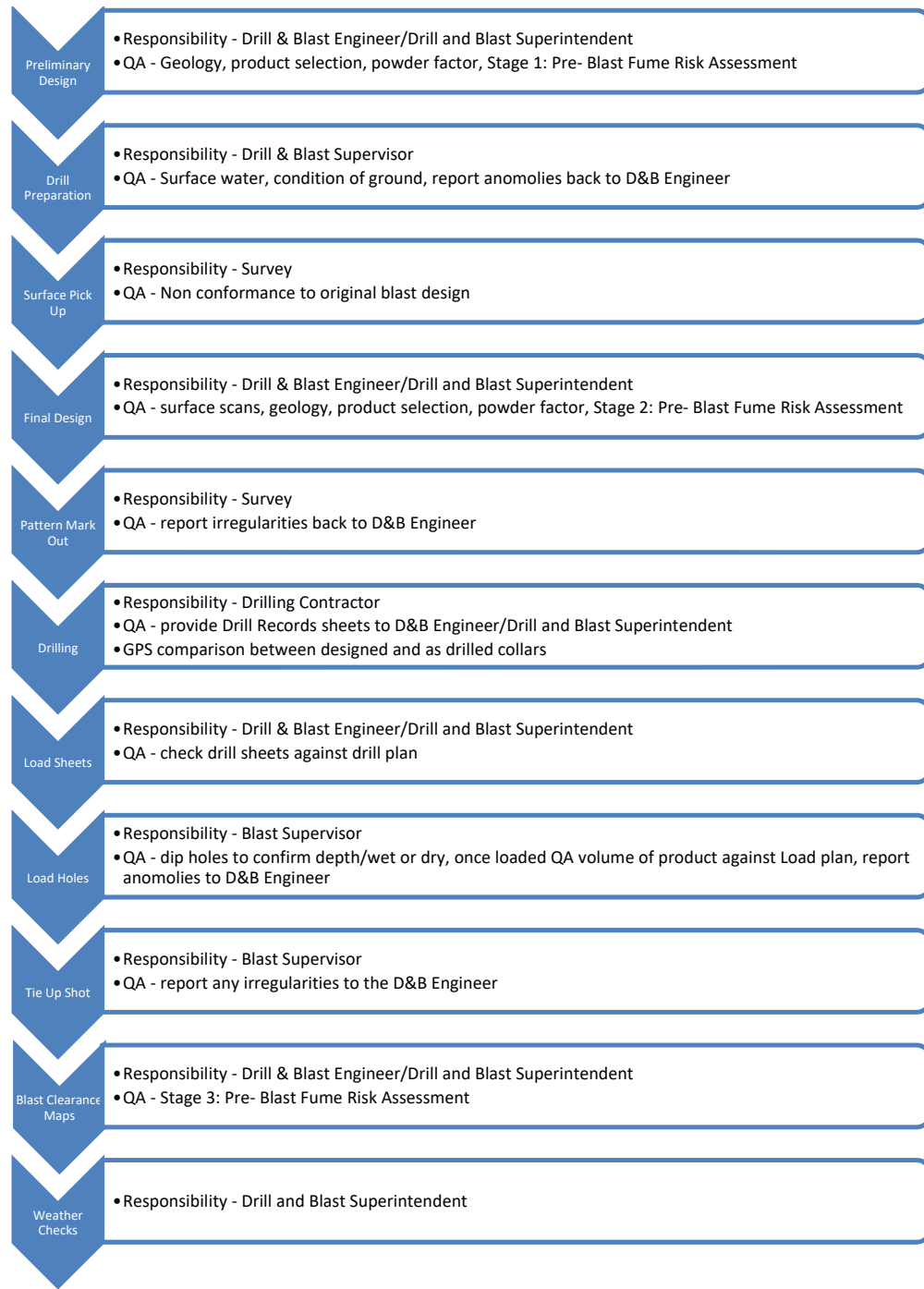
Figure 3: Blast Process Flowchart
