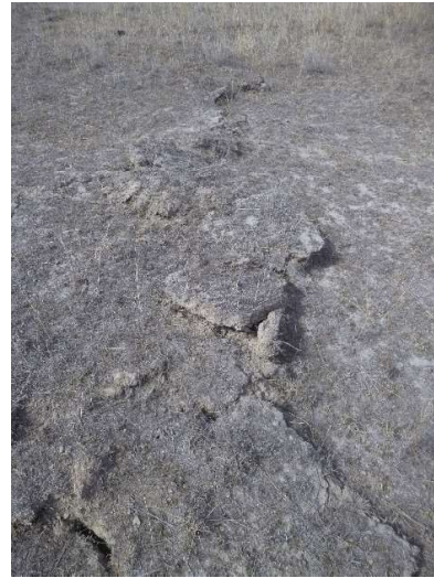
Fig. 4.5 Compression heaving above north-eastern end of WYLW17
