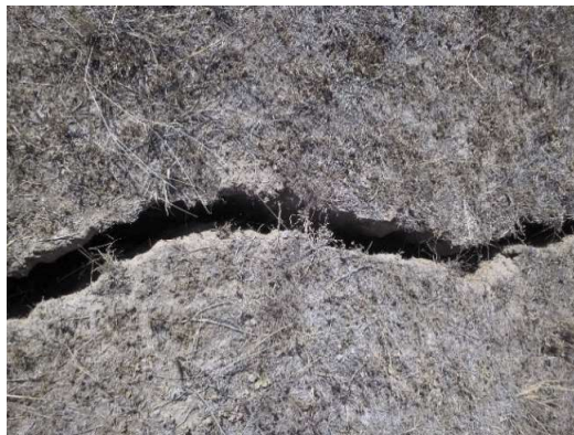
Fig. 4.4 Surface cracking above north-eastern end of WYLW17
