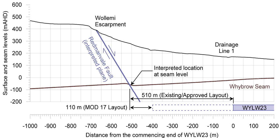
Fig. 1.6 Section through the Redmanvale Fault and the commencing end of WYLW23
