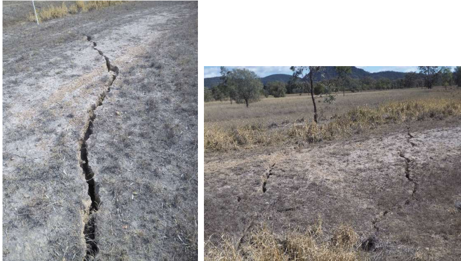
Fig. 4.7 Surface cracking above the middle of WYLW17
