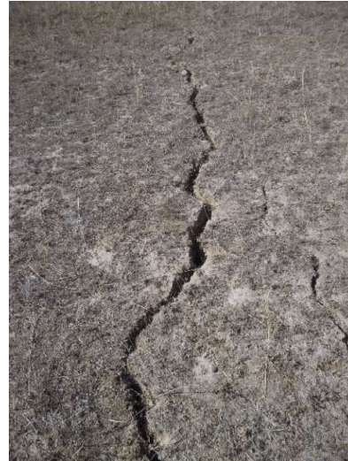
Fig. 4.4 Surface cracking above north-eastern end of WYLW17
