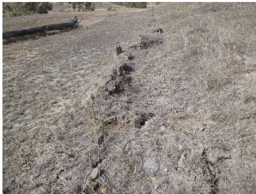
Fig. 4.5 Compression heaving above north-eastern end of WYLW17
