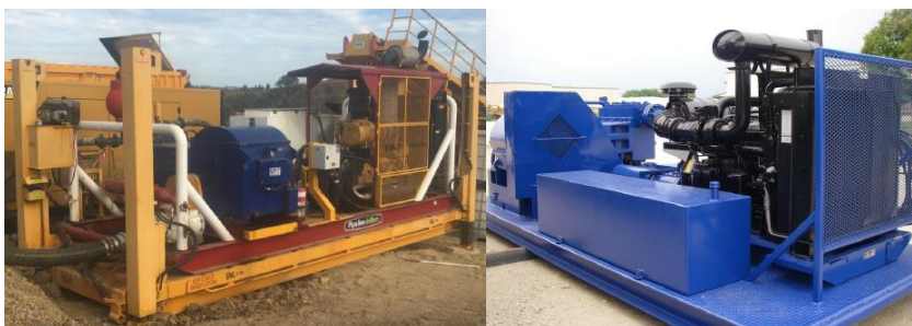
Figure 10: Example Mud Pump (refer to Project Technical Data Sheets)
