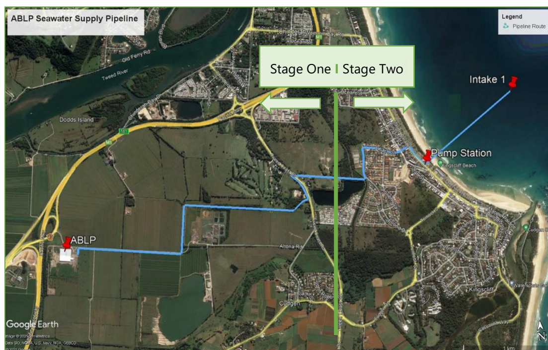
Figure 1.1: ABLP Seawater Supply Pipeline Alignment
