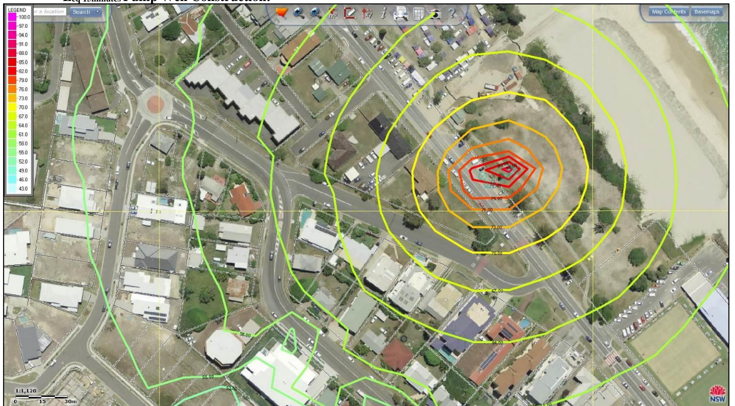
Leq 15minutes Pump Well Construction:
