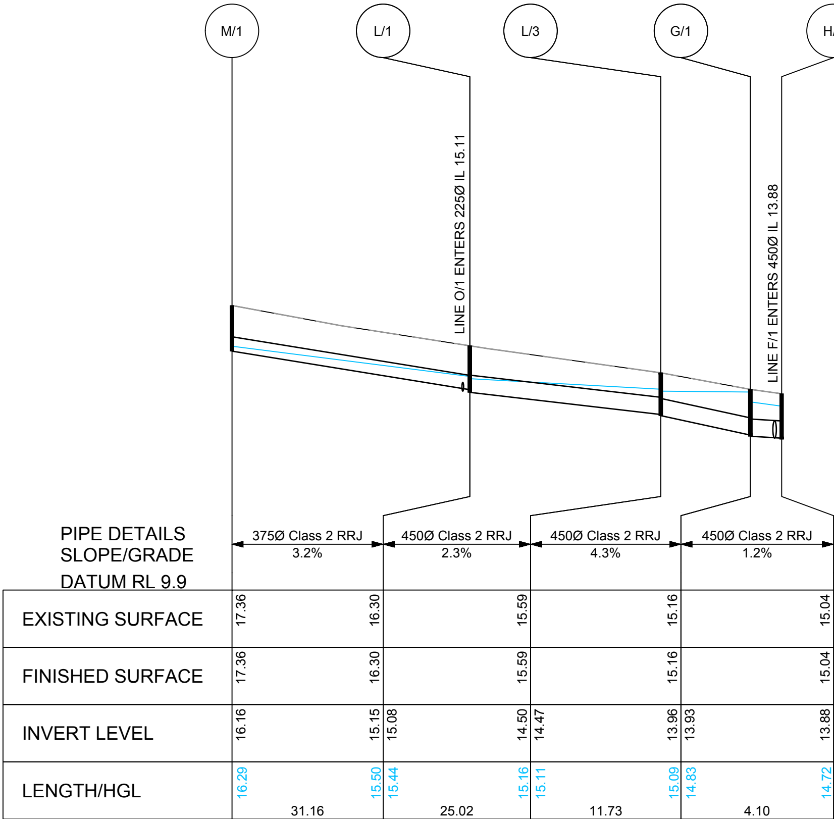
DRAINAGE LONGITUDINAL SECTION FOR LINE M/1 - H/1 SCALES: HORIZONTAL 1:500 VERTICAL 1:100
