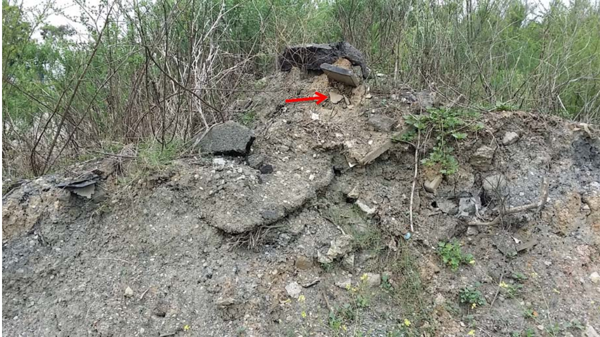
Photograph No. 7: Fragment of asbestos cement sheet that was removed from the soil in the north east area of the stockpile
