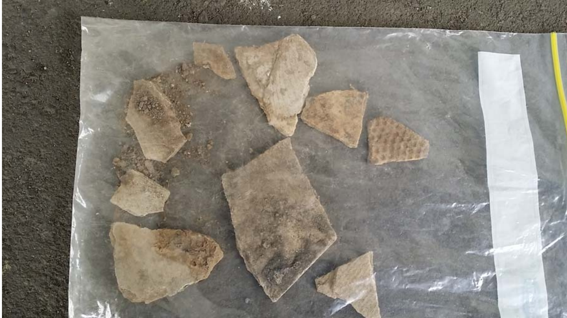
Photograph No. 9: Fragments of asbestos cement sheet debris collected on 9 December 2013 from the soil stockpile in the north western area of the Yennora Distribution Centre
