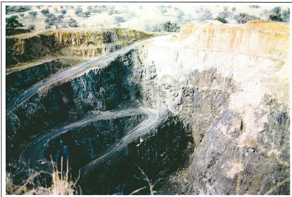
Plate 2.2 Existing Bald Hill Quarry void access road (Ref: 509B/23)
