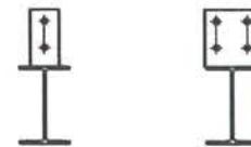
TYPICAL PURLIN & GIRT CLEATS ALL CLEATS FROM 8mm PLATE ALL BOLTS M12
