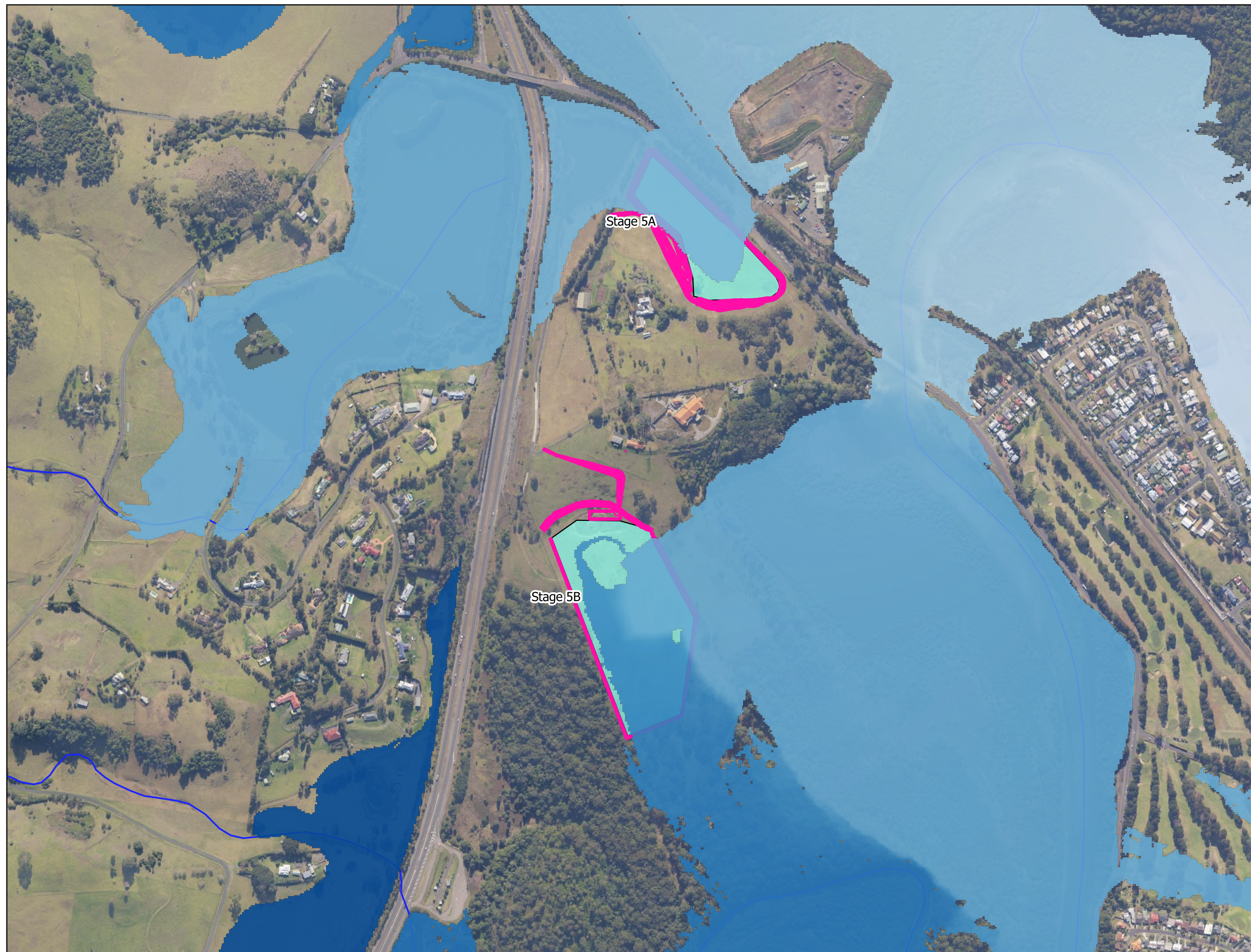
FIG 3. 1% AEP Flood height, existing conditions.
