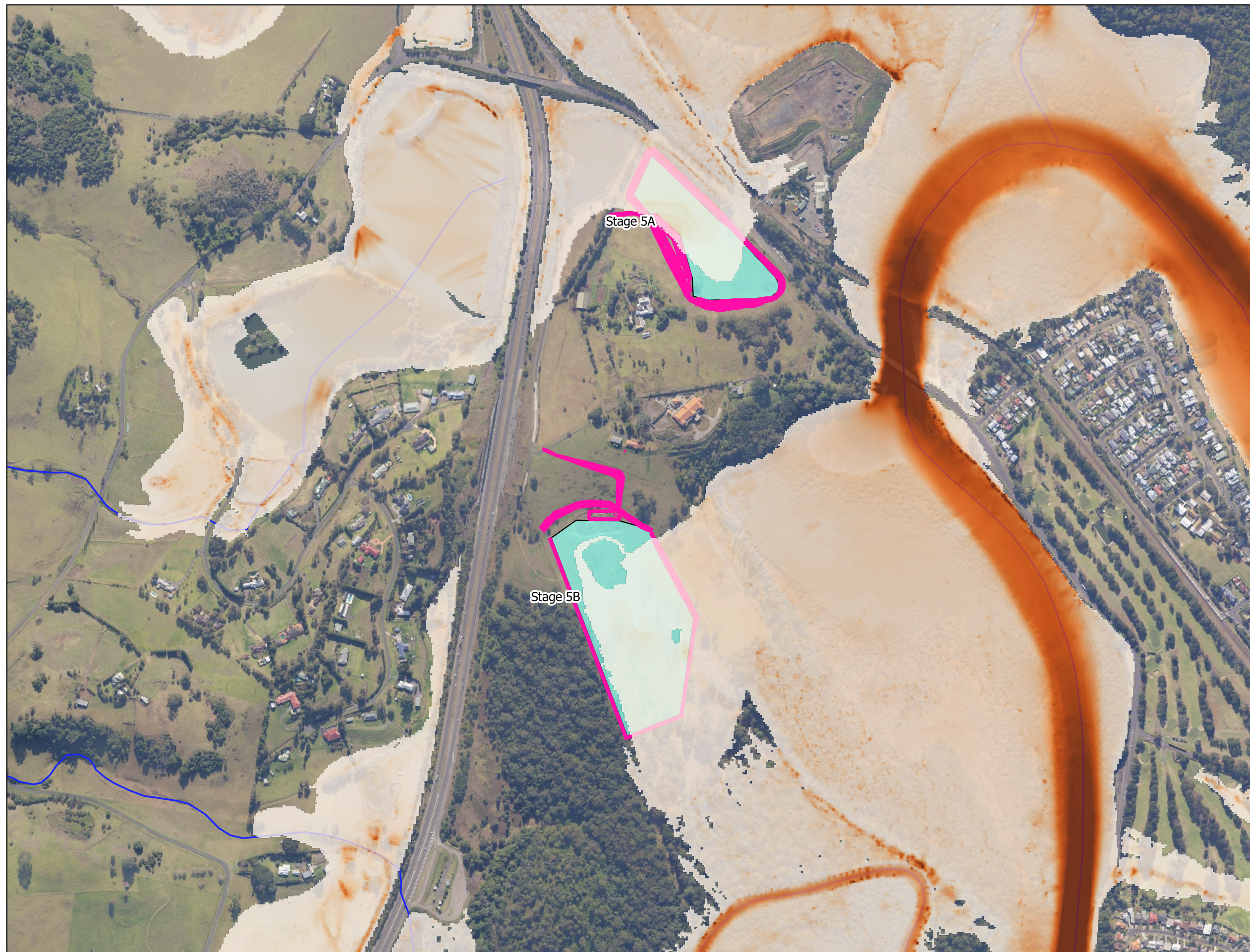
FIG 5. 100y ARI Max velocity, existing conditions.
