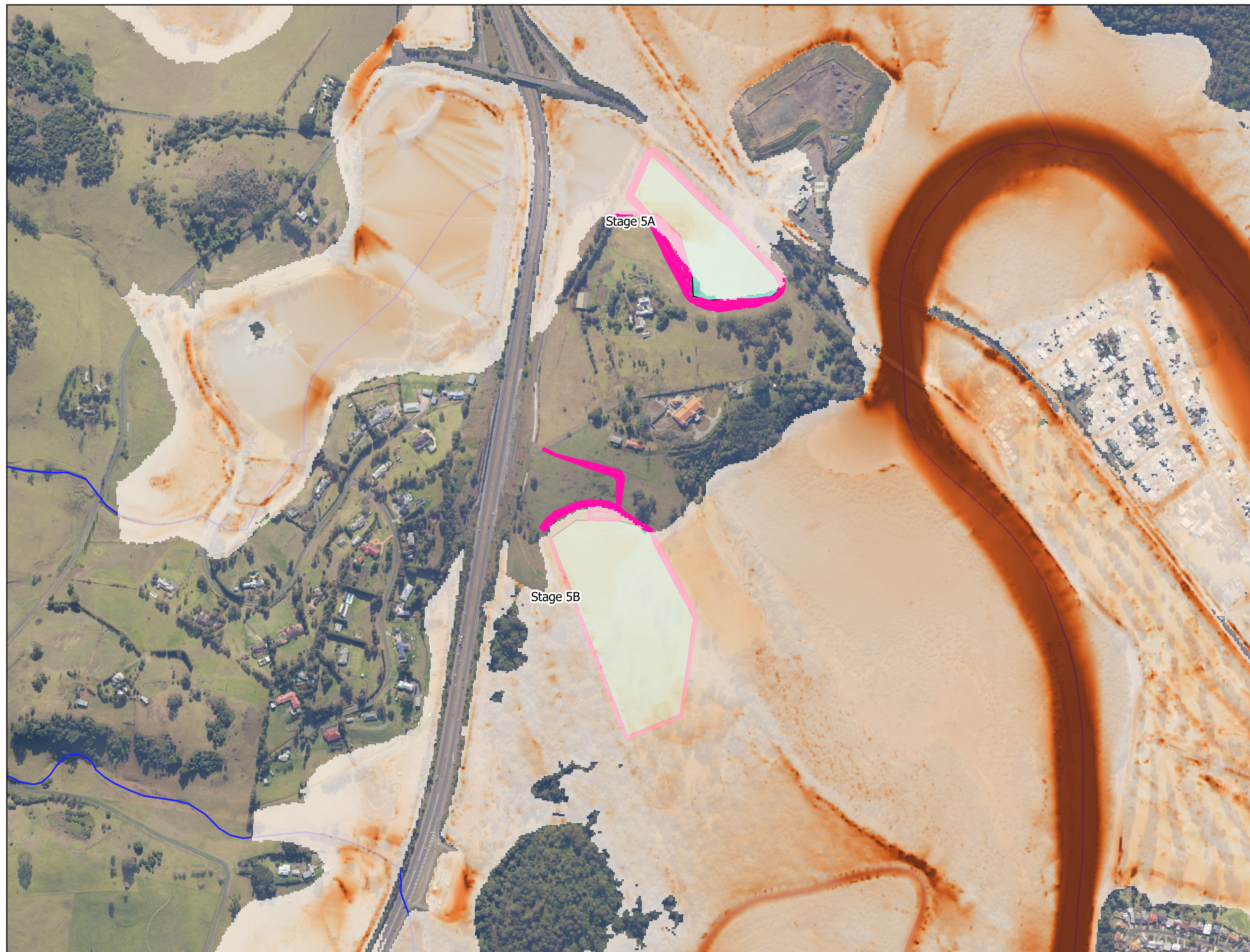
FIG 6. PMF Max velocity, existing conditions.
