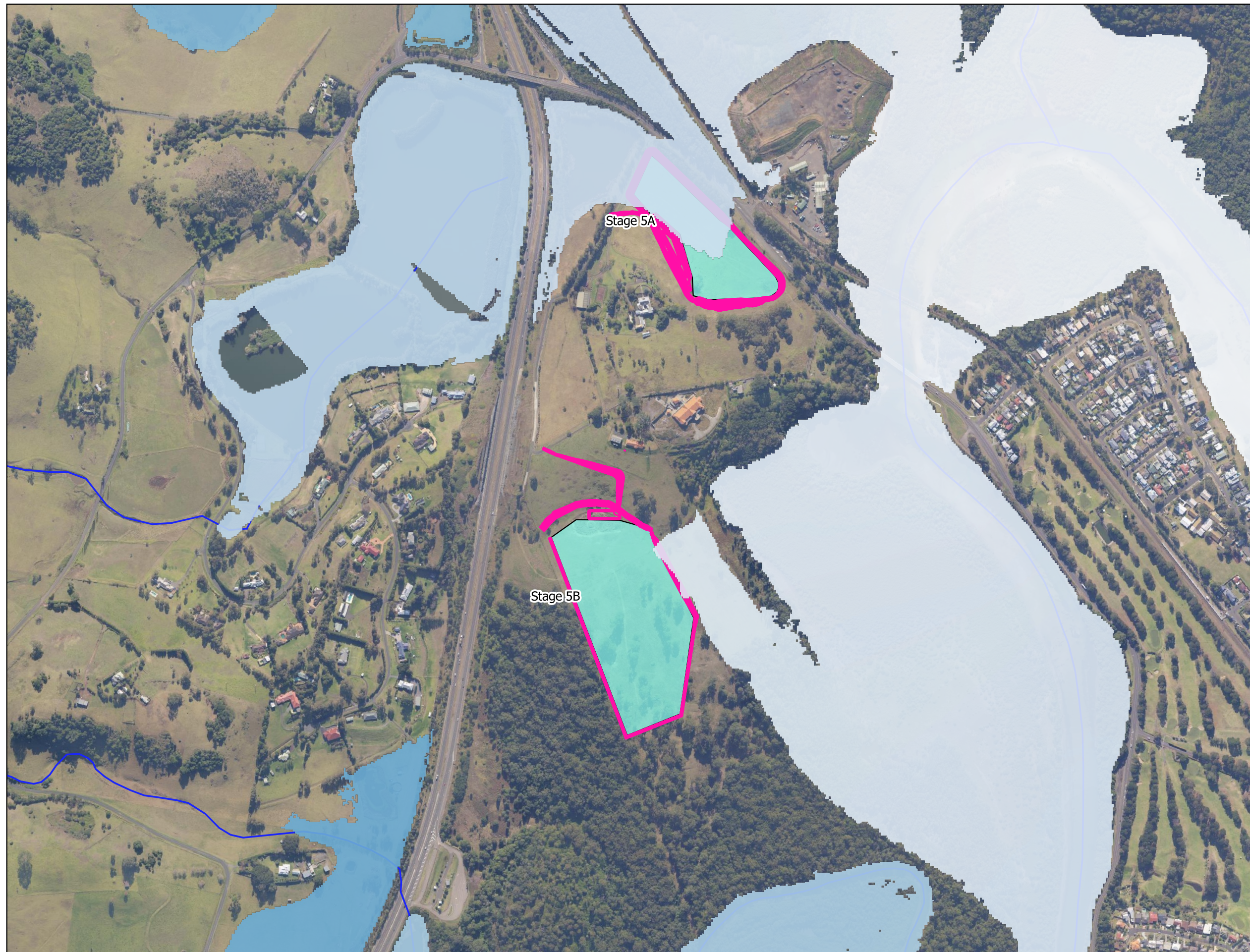
FIG 1. 5y ARI Flood height, existing conditions.
