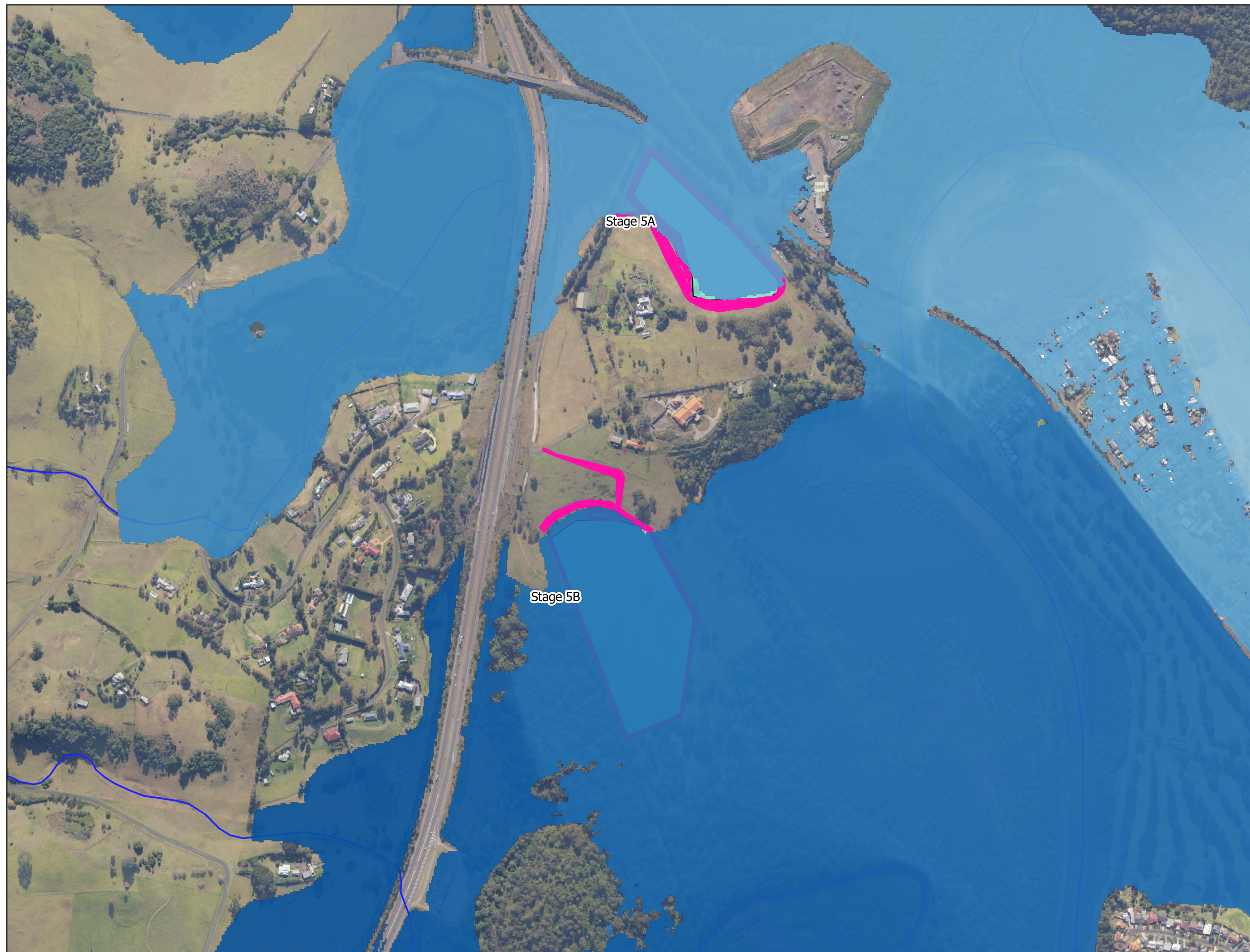
FIG 4. PMF Flood height, existing conditions.
