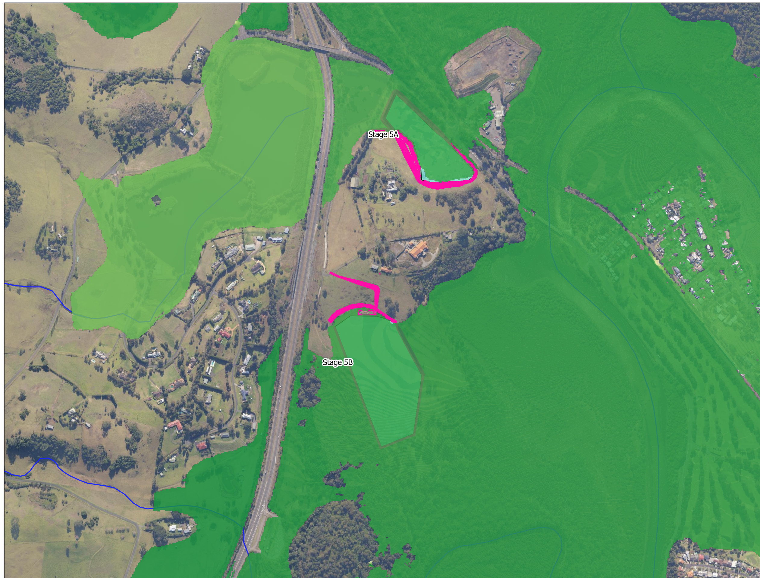
FIG 10. PMF Flood height difference
