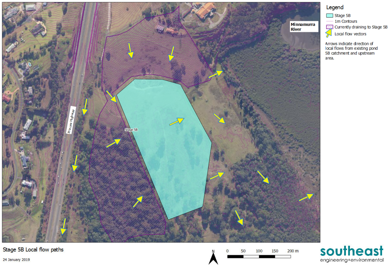
Figure 3.4 Surface flows around Stage 5B
