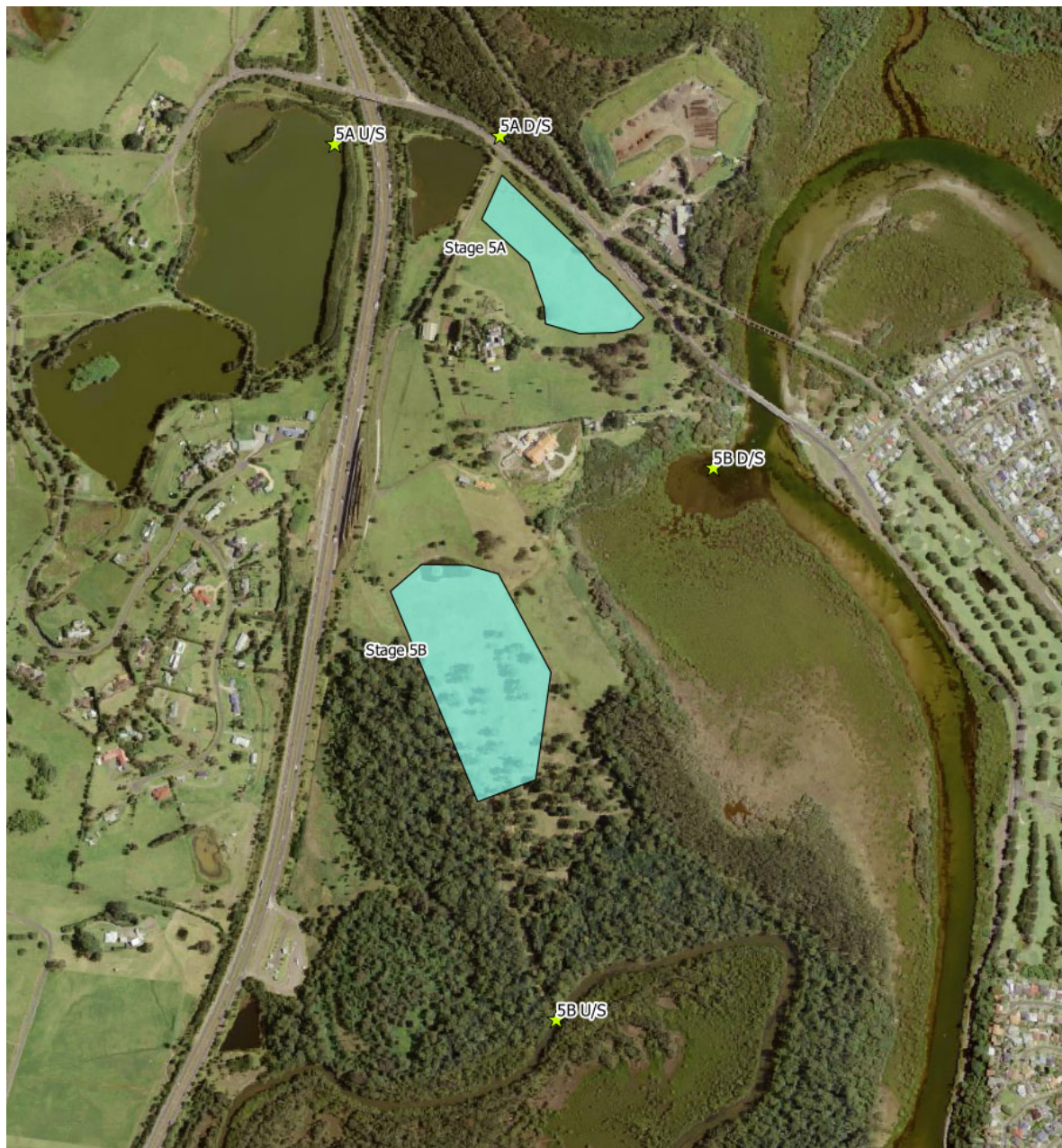
Figure 4.6 Proposed water quality monitoring points upstream (U/S) and downstream (D/S) of Stage 5A and 5B extraction areas.
