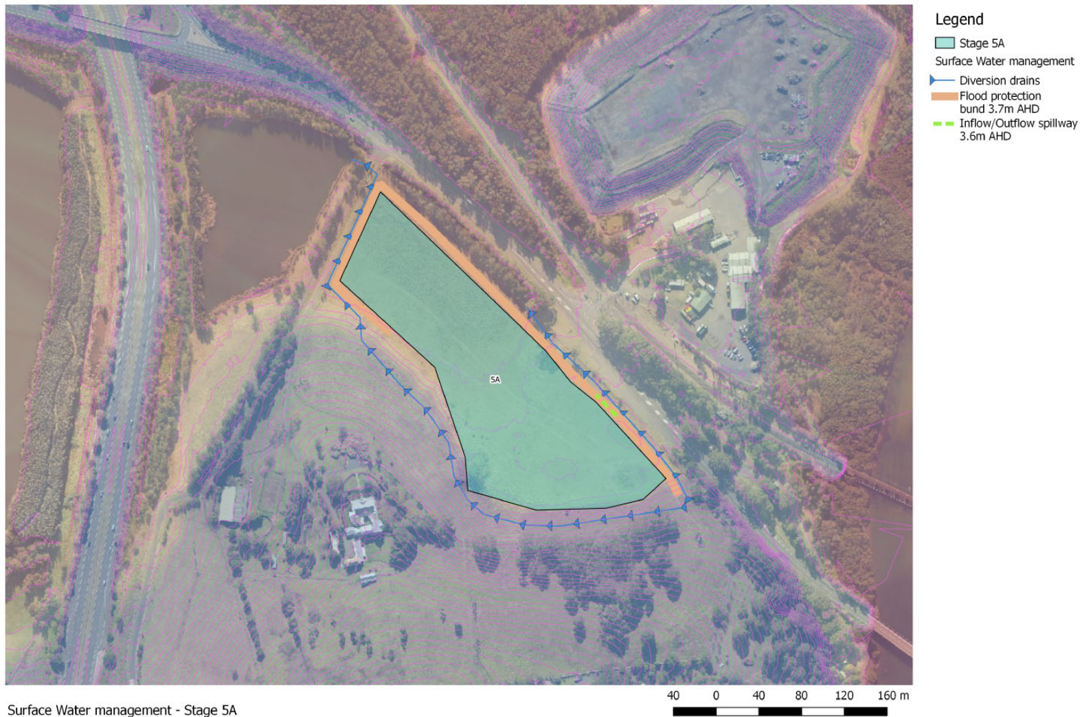
Surface Water management - Stage 5A
