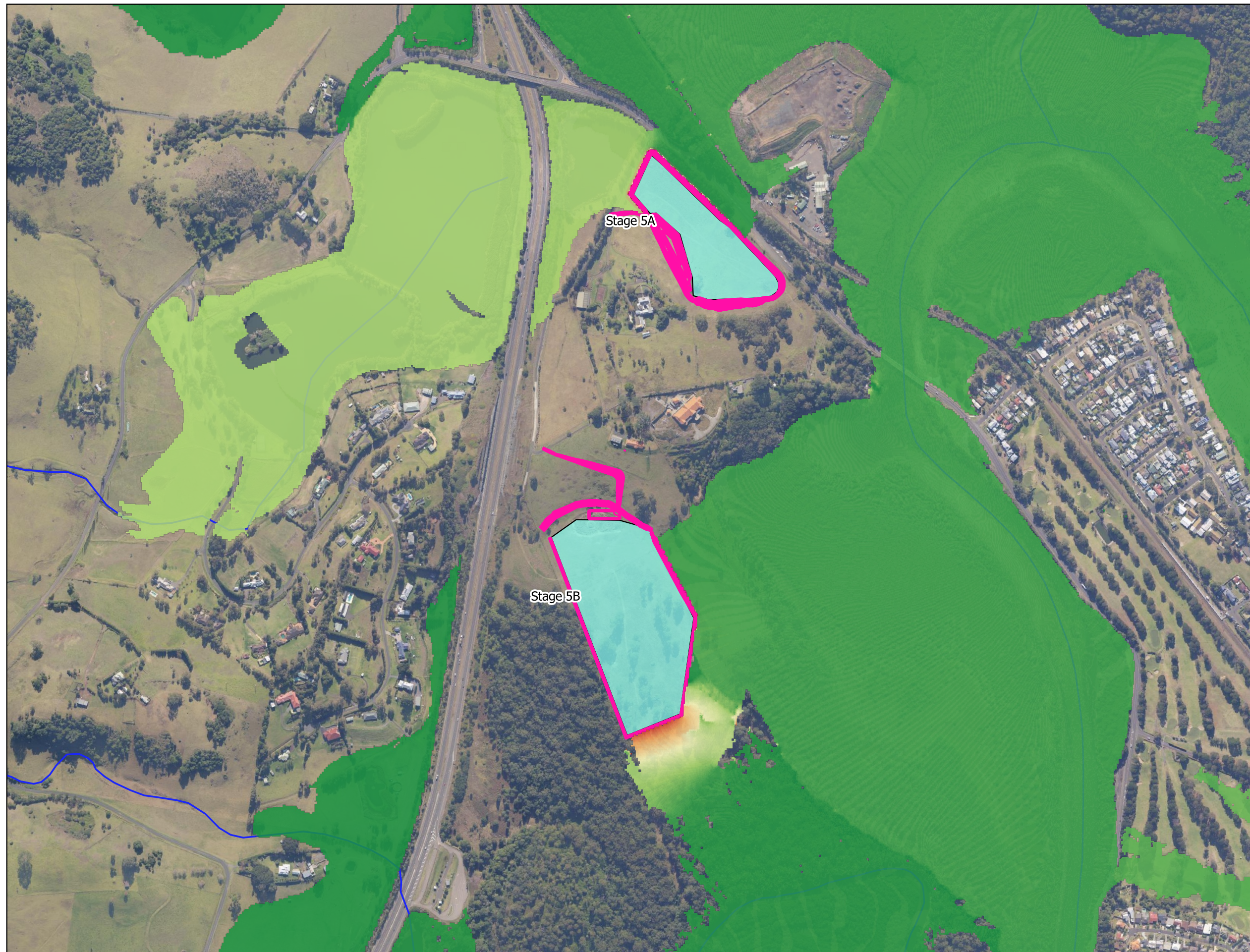
FIG 9. 100y ARI Flood height difference
