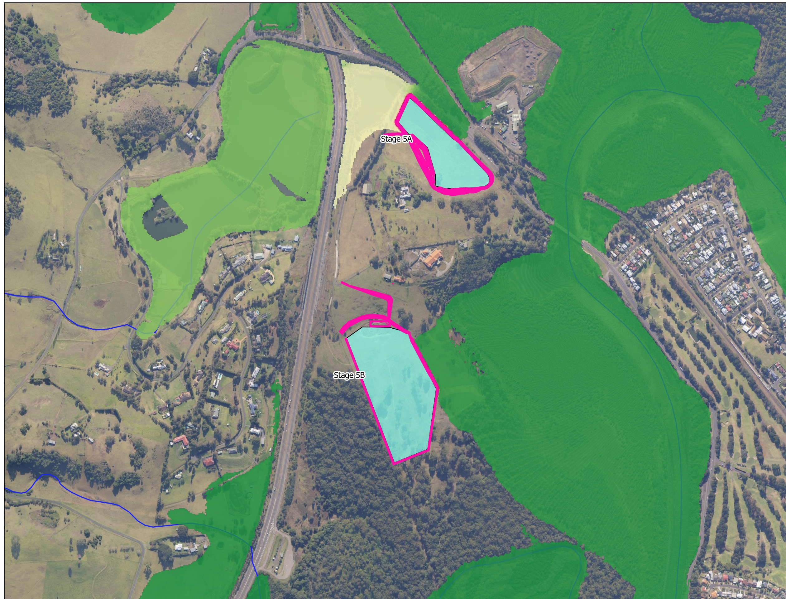
FIG 8. 20y ARI Flood height difference
