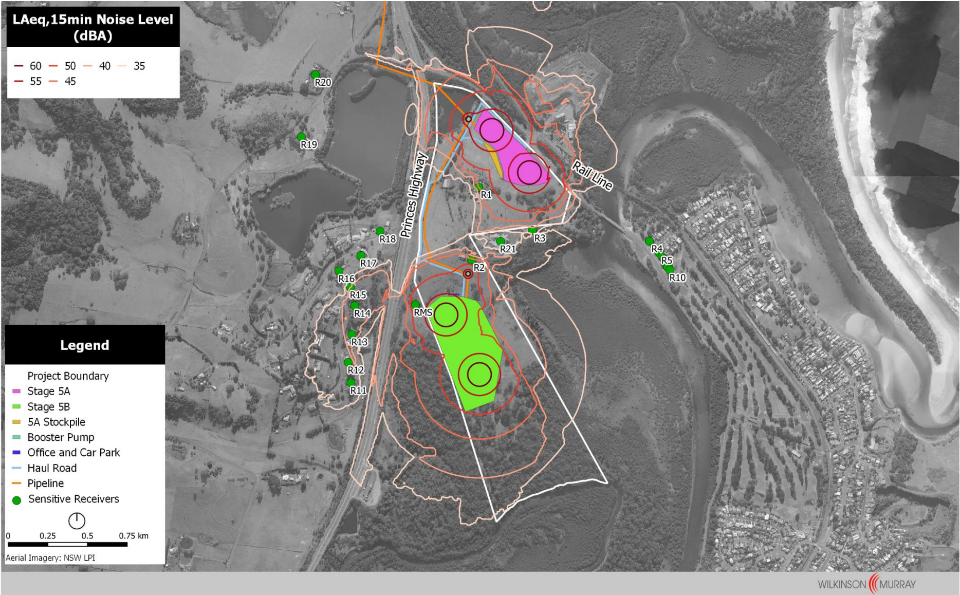
Figure A-2 LAeq,15min Noise Levels – AM Shoulder, Temperature Inversion
