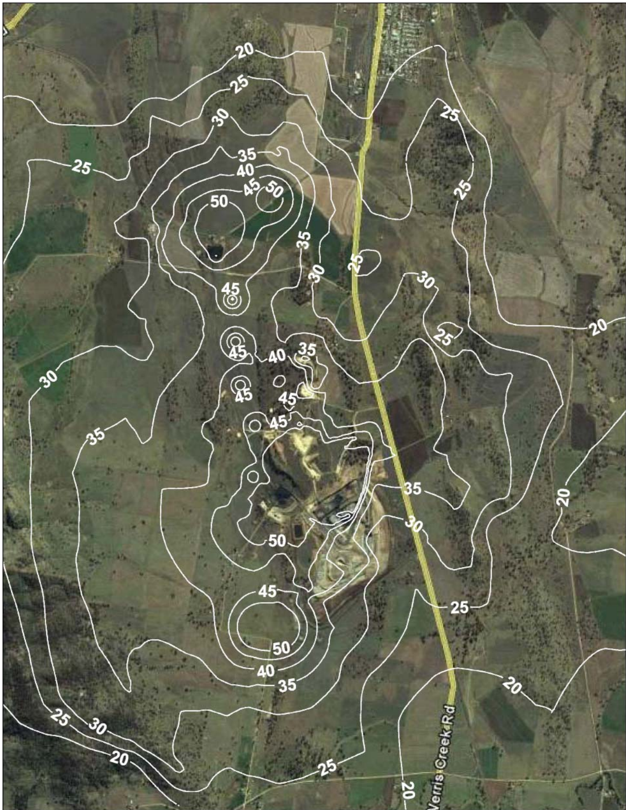
Figure B1. Predicted Scenario 1 noise contours dB(A), L_{eq(15min)} – Neutral atmosphere
