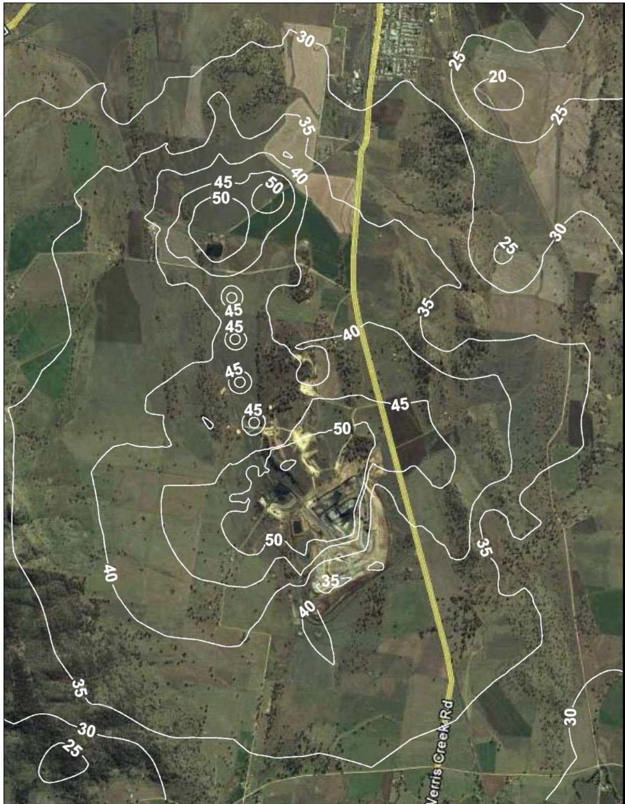
Figure B2. Predicted Scenario 1 noise contours dB(A), L_{eq}(15min) – Inversion
