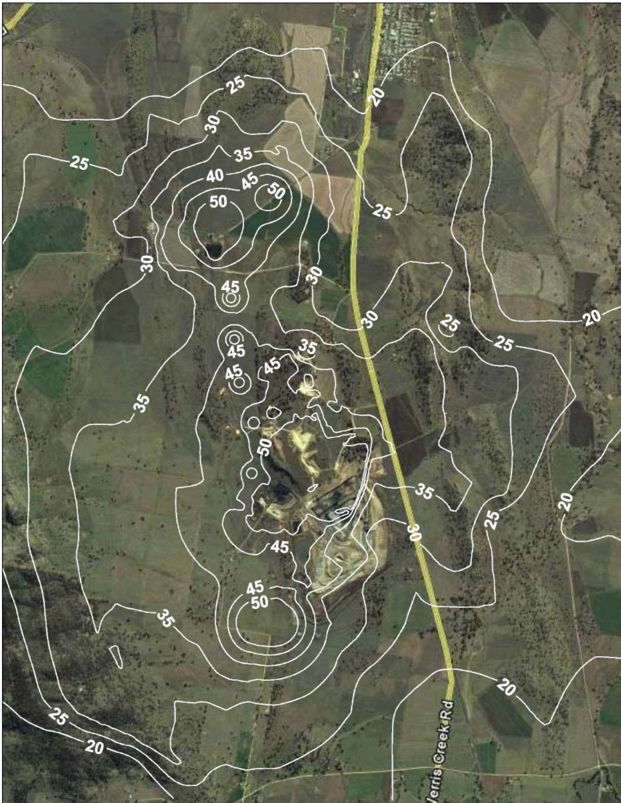
Figure B3. Predicted Scenario 2 noise contours dB(A), L_{eq(15min)} – Neutral atmosphere
