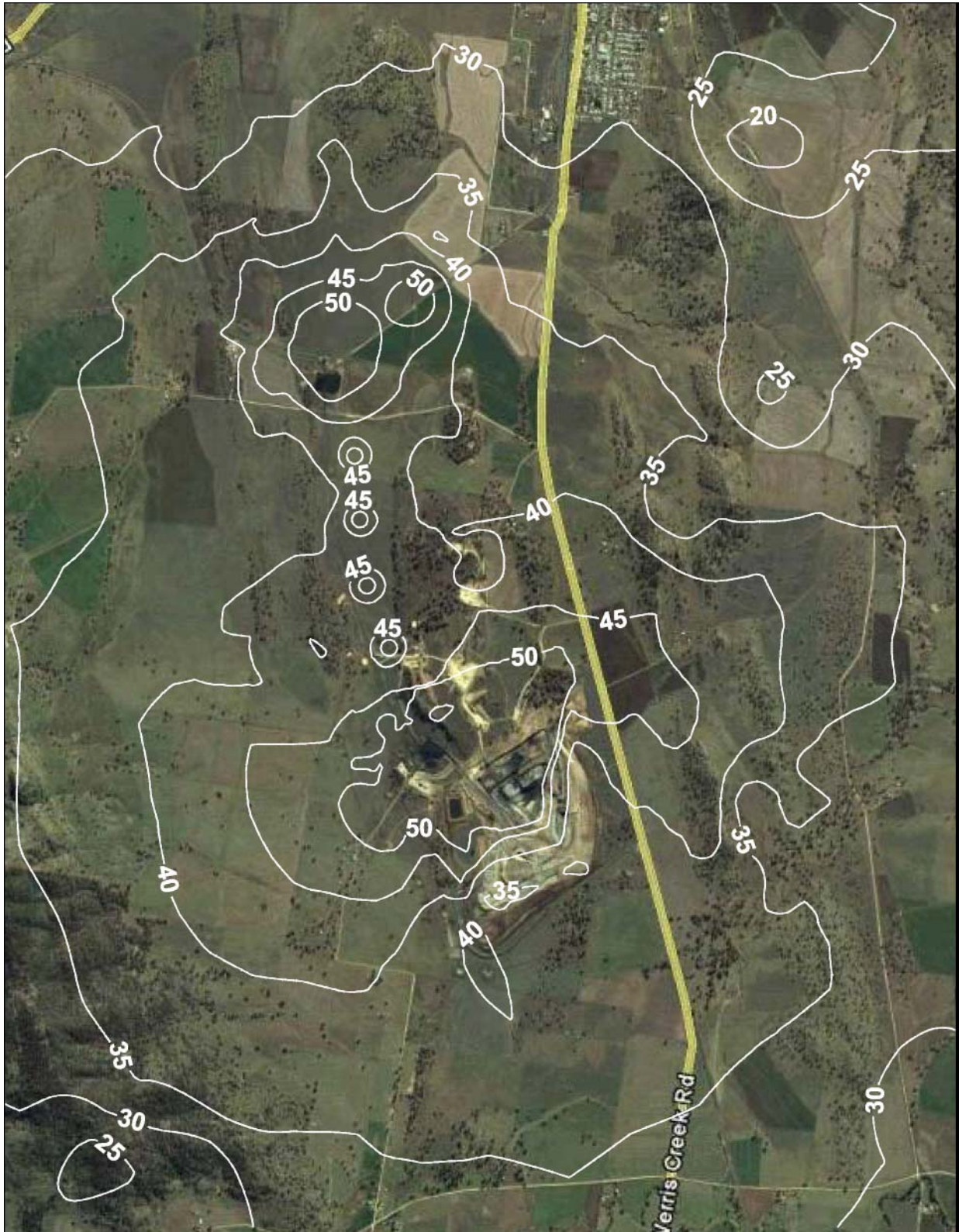
Figure B6. Predicted Scenario 3 noise contours dB(A), L_{eq}(15min) – Inversion
